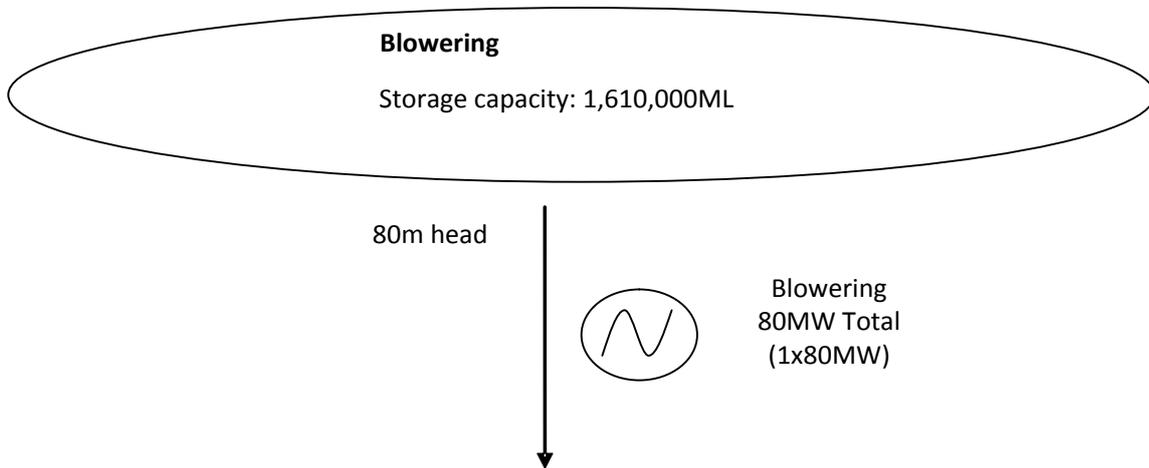
Figure 13 Hume power station hydro model
