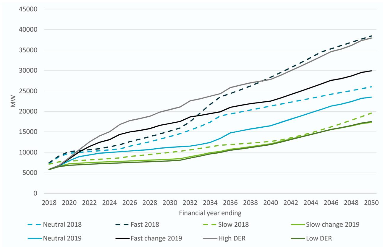
Figure 5-1: Residential rooftop solar capacity by scenario
