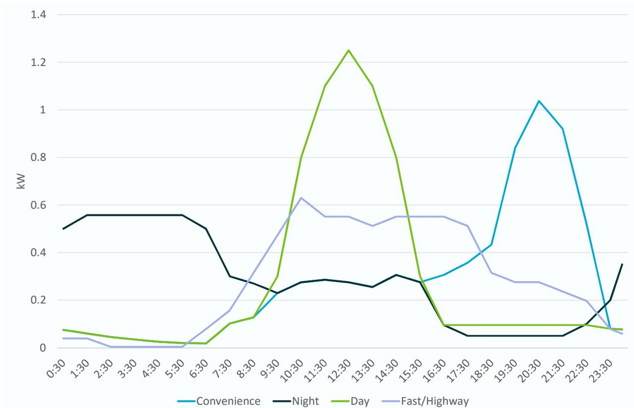
**Figure 5-18: Passenger electric vehicle charging profiles (national annual average daily basis)**
