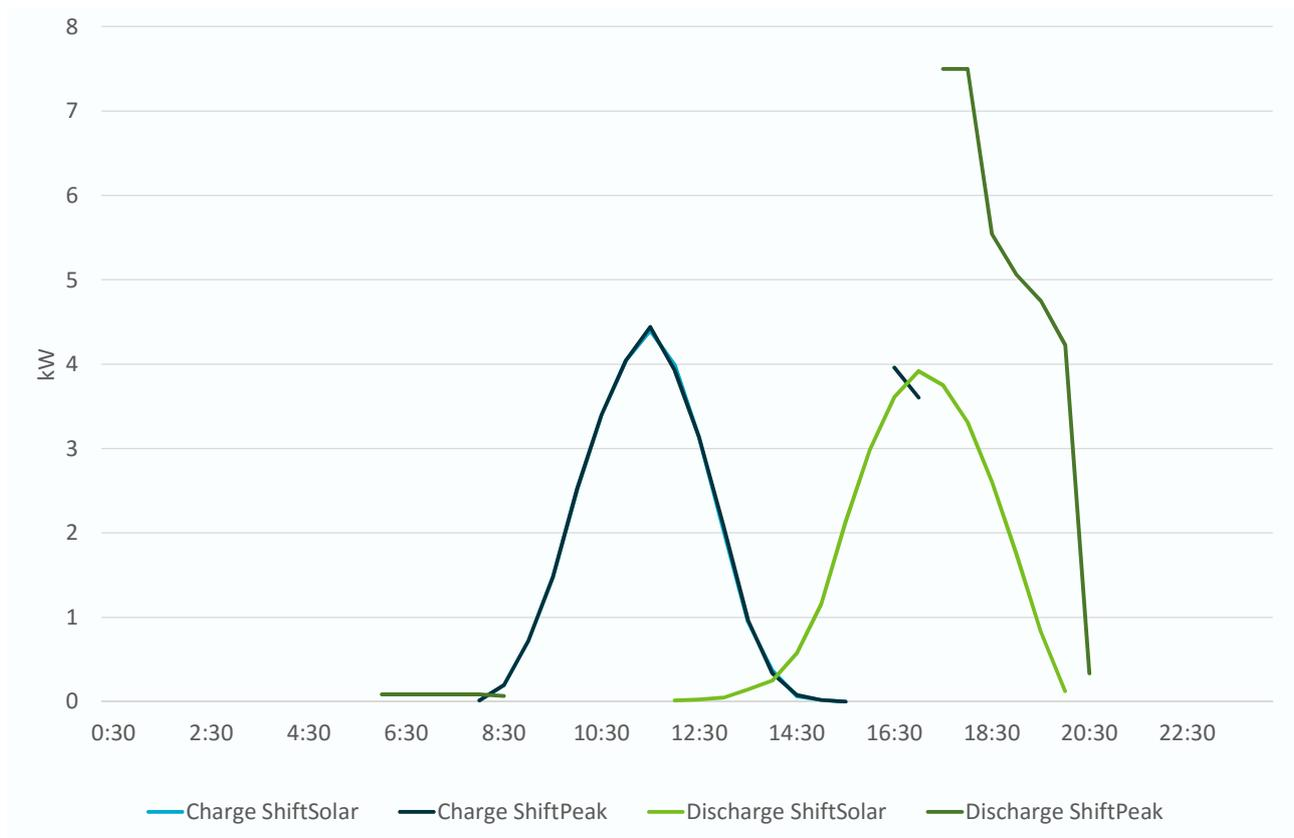
**Figure 5-22: Average commercial battery storage profiles (half hour ending, average of 90 days over summer period)**
