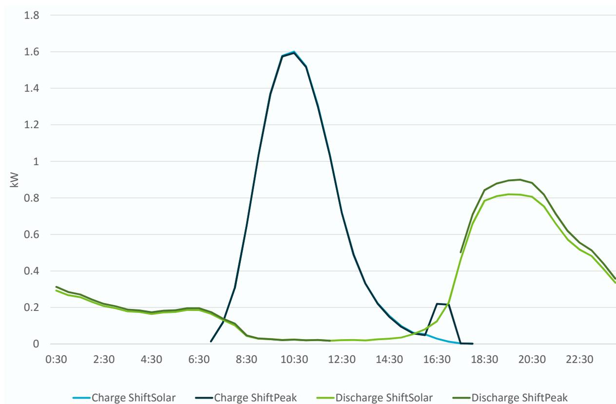
**Figure 5-21: Average residential battery storage profiles (half hour ending, average of 90 days over summer period)**
