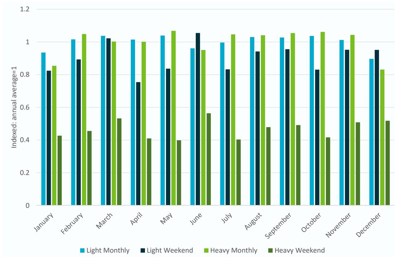
Figure 5-17: Factors for adjusting light and heavy vehicle charging profiles for month and weekend.
