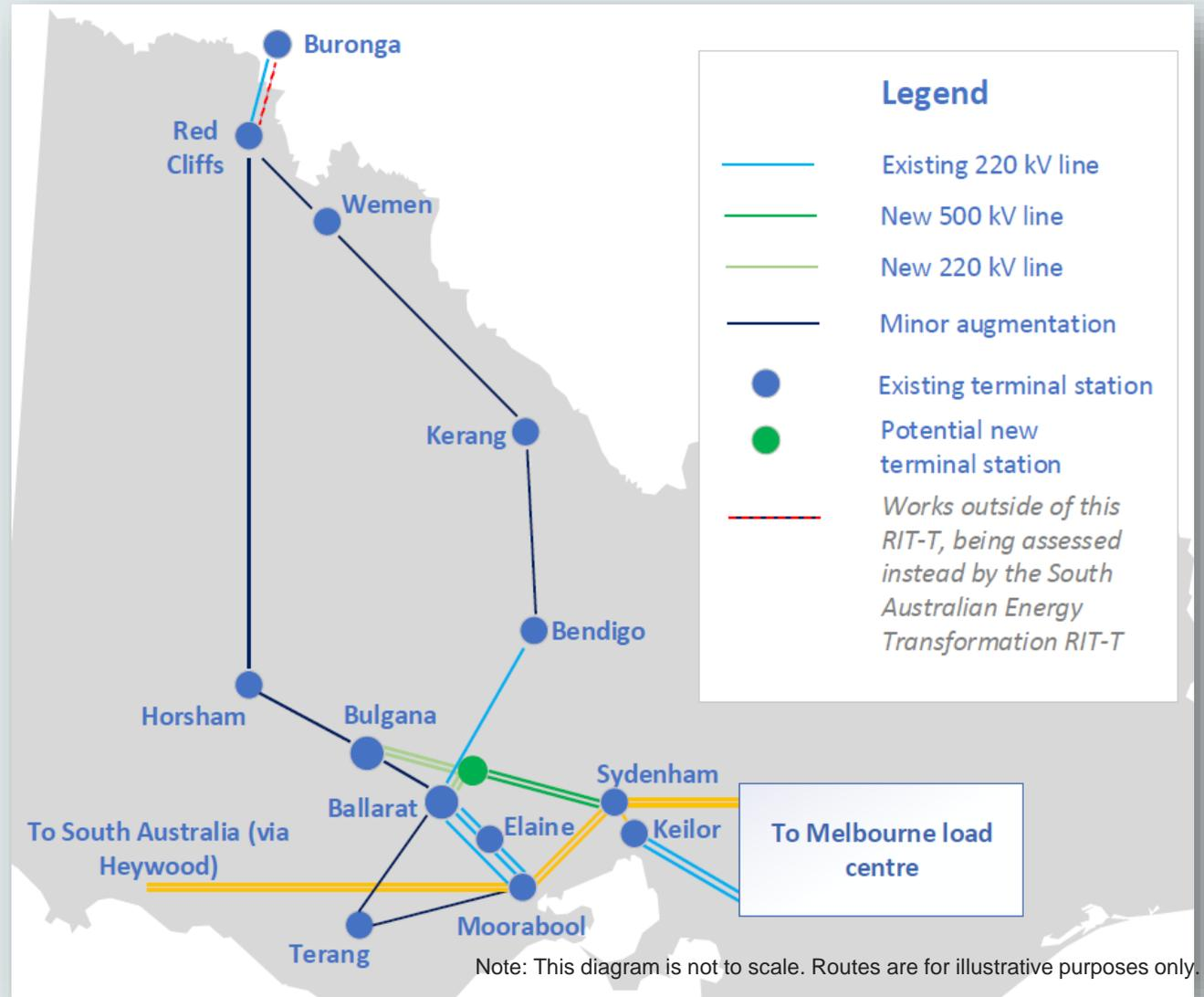
1. Initial assessment has indicated that there may be insufficient space in Ballarat Terminal Station for the proposed 500 kV plant. AEMO has assumed that a new terminal station will be established close to Ballarat with connections back to the existing Ballarat Terminal Station in its assessments.
