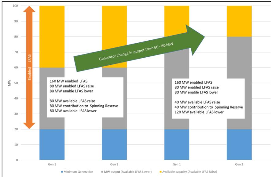
In the example shown in Figure 4, two generators generate 60 MW each. They provide LFAS and contribute 80 MW to Spinning Reserve. If their output increases, the LFAS enablement stays the same. However, the contribution to Spinning Reserve between the two generators drops to 40 MW. If this change persisted, additional Spinning Reserve would need to be made available, potentially by bringing on another generator. If enabled, this generator could also then provide LFAS.
