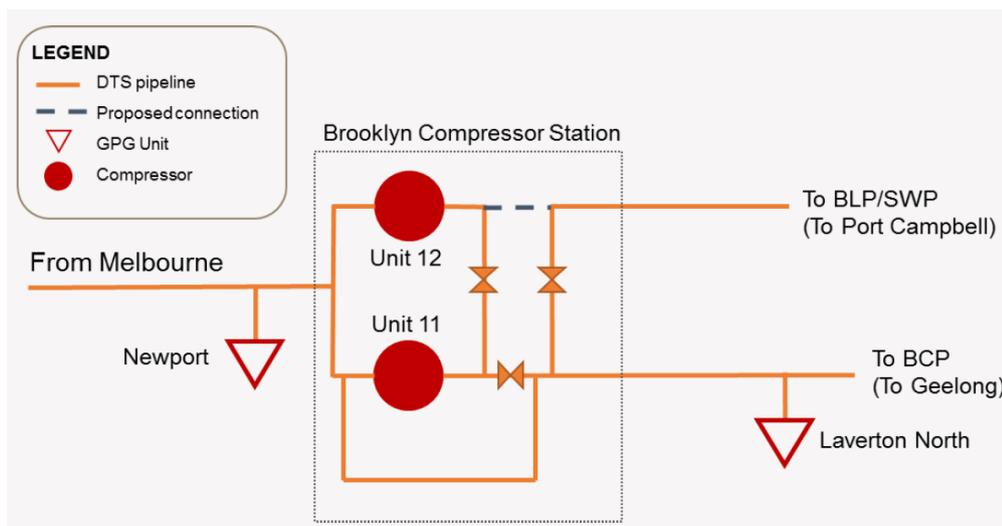
Figure 2: Simple flow diagram of Brooklyn Compressor Station
