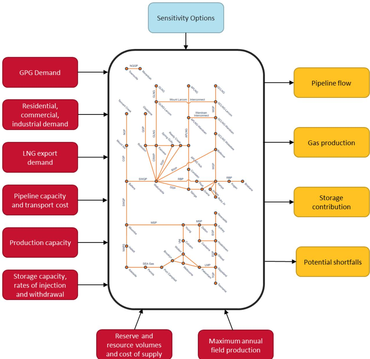
The eastern and south-eastern gas network is represented by a series of connected nodes. At each node, gas may be injected into or withdrawn from the network where production facilities and loads are connected respectively.
