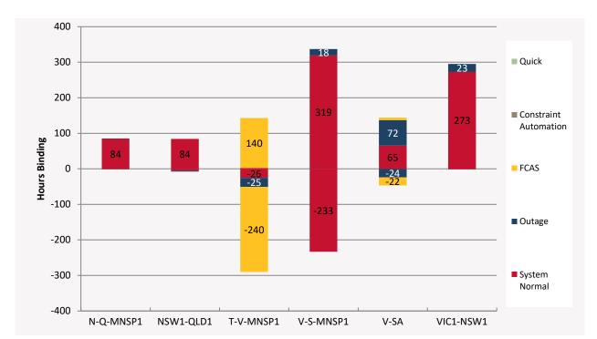
Figure 1 Interconnector binding dispatch hours
