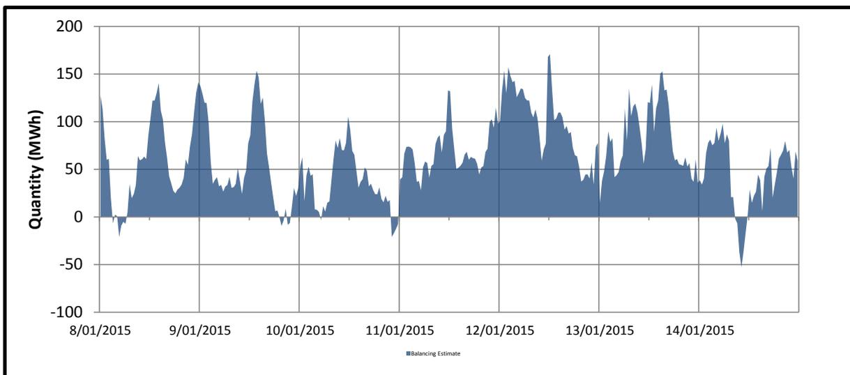
The majority of the balancing activity this week occurred within Balancing Demand. The maximum balancing demand for the week reached 170.7165 MWh on the 12/1/2015. The maximum balancing supply for the week reached -52.834 MWh on the 14/1/2012.
