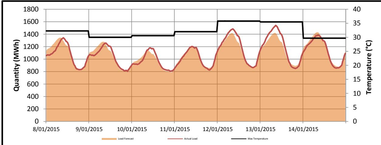
The maximum temperatures for this trading week ranged from 29.7°C to 35.8°C. The actual load peaked at 1541.795 MWh on the 13/1/2015.
