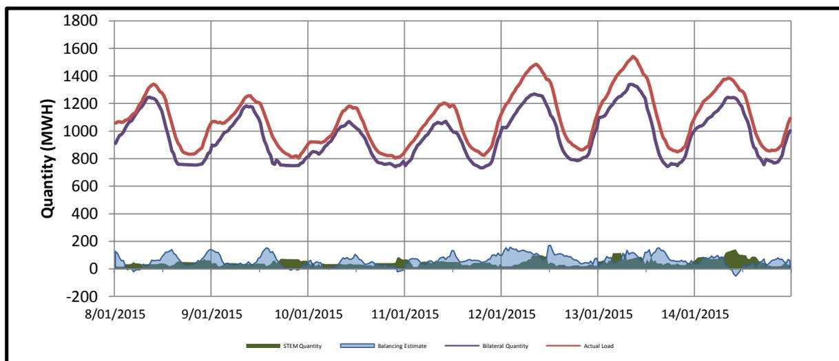
Total balancing supply equalled -291.87 MWh whereas total balancing demand equalled 21561.533 MWh. The Total STEM Traded quantity was 16251.994 MWh, with the STEM Clearing Quantity ranging between 13.33 MWh and 142.072 MWh.
