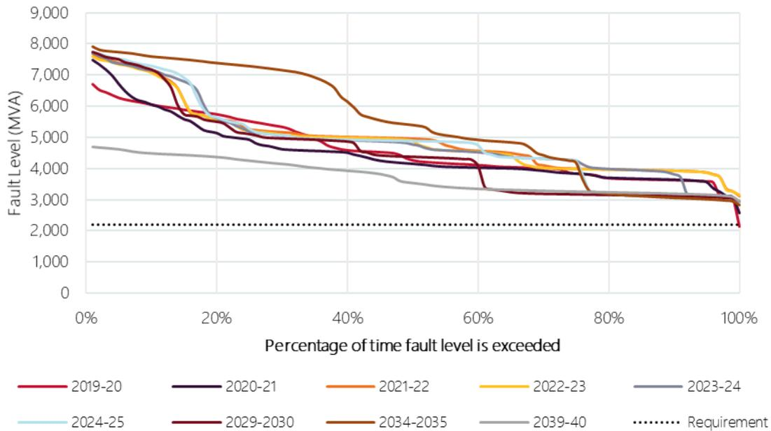
**Figure 166 Projected Robertstown 275 kV fault level duration curves**
