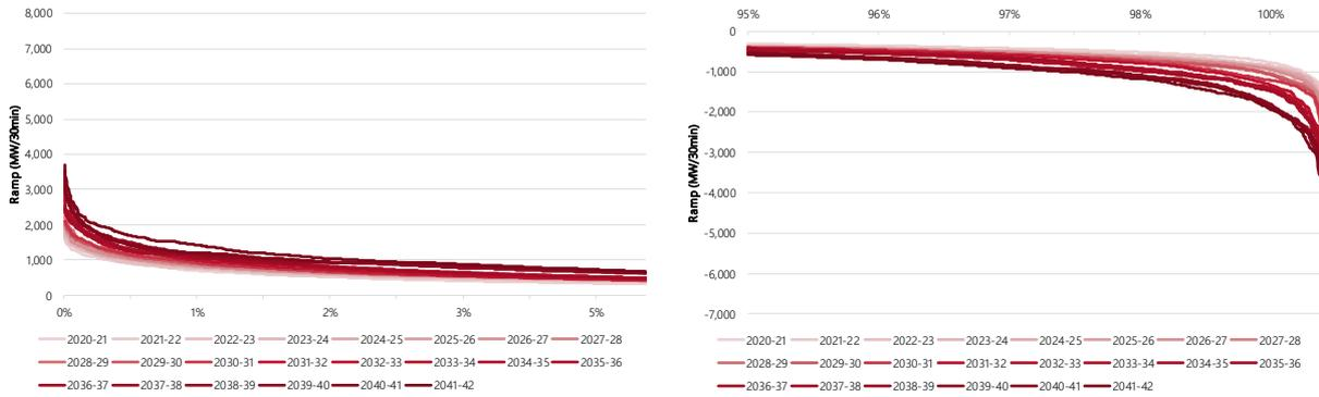
**Figure 59 Forecast top 5% and bottom 5% of ramp events in South Australia from dispatchable generators by financial year to 2041-42**
