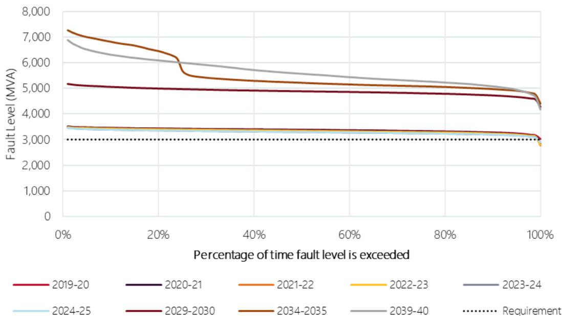
**Figure 153 Projected Sydney West 330 kV fault level duration curves**
