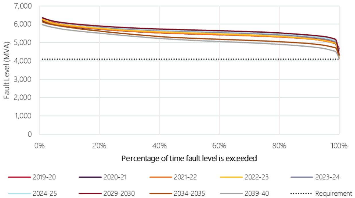
**Figure 176 Projected Moorabool 220 kV fault level duration curves**
