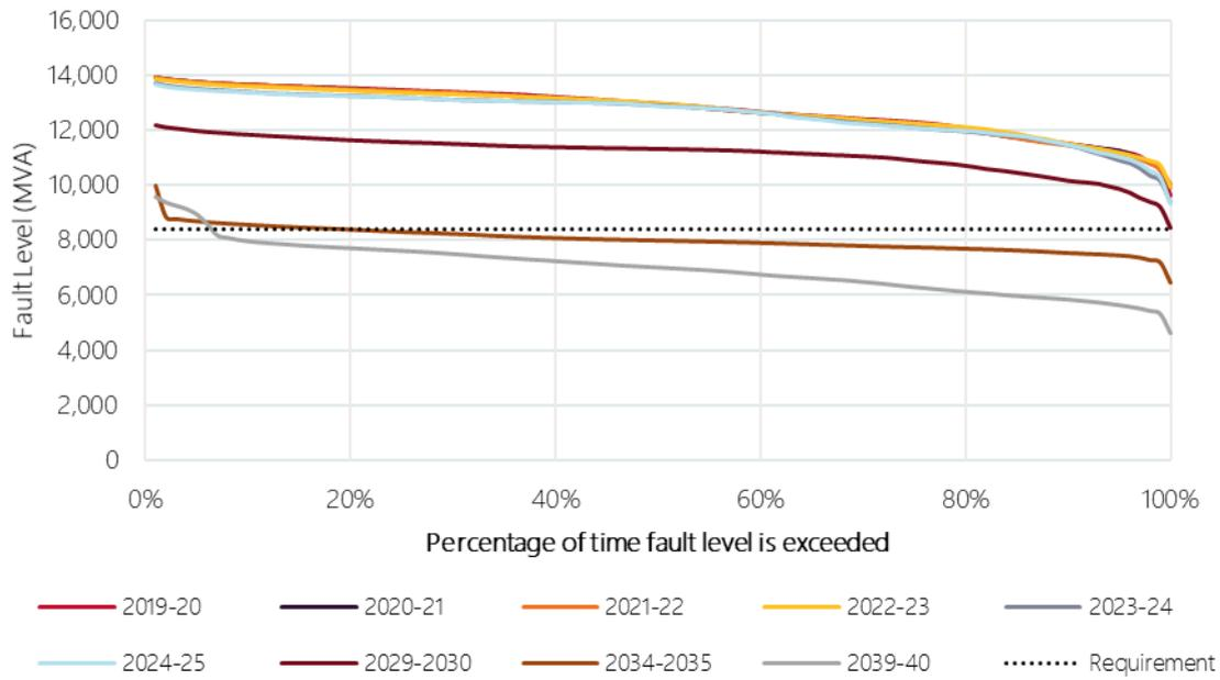
**Figure 156 Projected Darlington Point 330 kV fault level duration curves**
