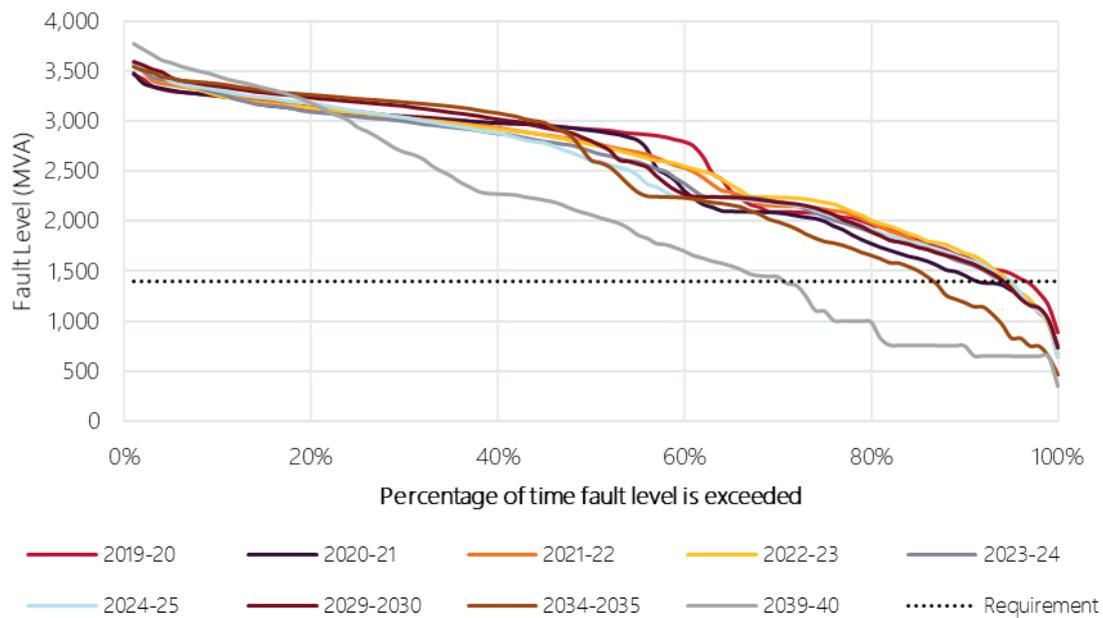
**Figure 171 Projected Burnie 110 kV fault level duration curves**
