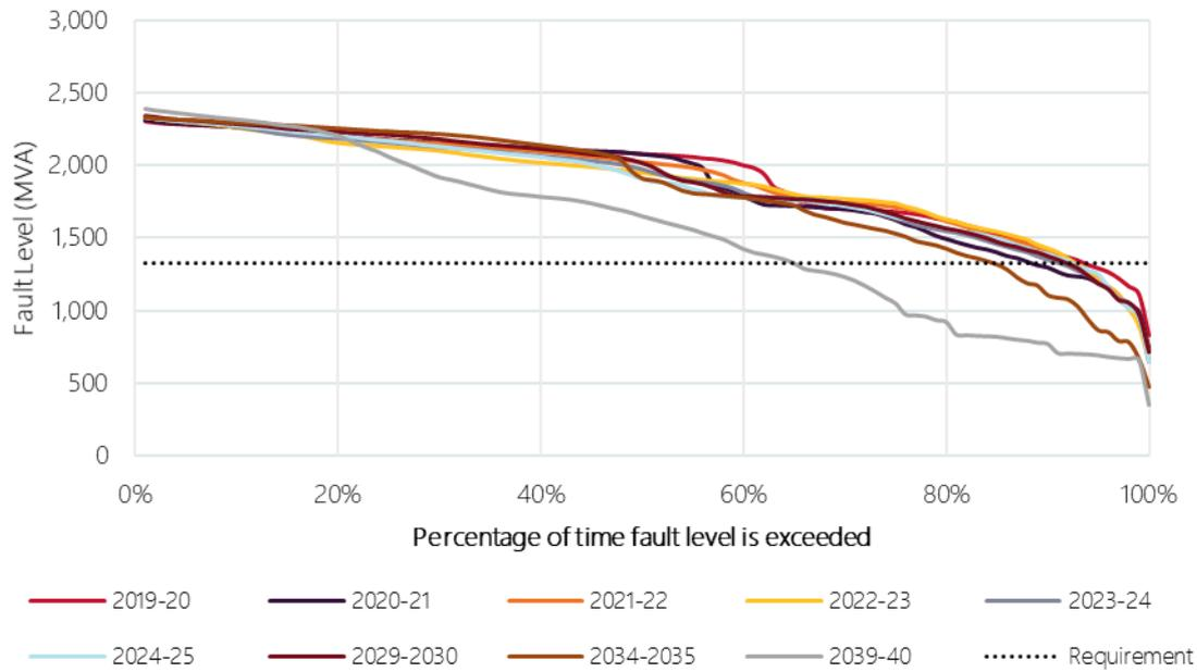
**Figure 170 Projected Waddamana 220 kV fault level duration curves**
