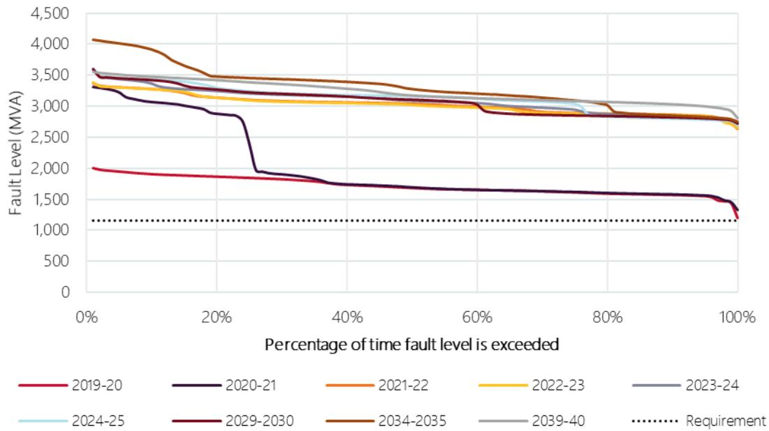
**Figure 165 Projected Para 275 kV fault level duration curves**
