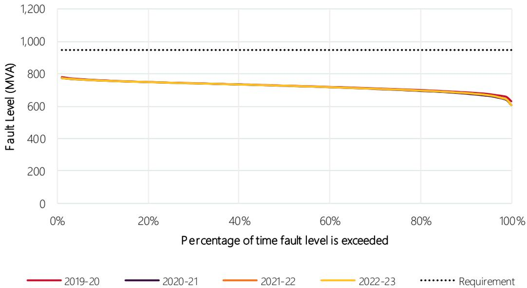
**Figure 174 Projected Red Cliffs 220 kV fault level duration curves, including after Project EnergyConnect commissioning**
