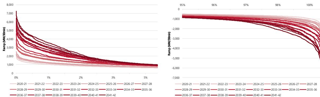
**Figure 57 Forecast top 5% and bottom 5% of ramp events in Queensland from dispatchable generators by financial year to 2041-42**
