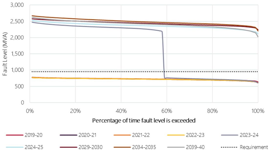
**Figure 175 Projected Thomastown 220 kV fault level duration curves**
