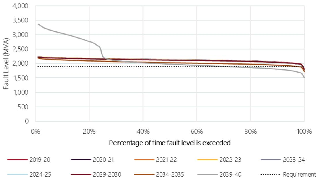
**Figure 155 Projected Newcastle 330 kV fault level duration curves**
