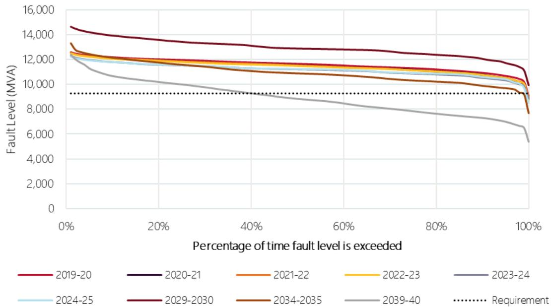
**Figure 154 Projected Wellington 330 kV fault level duration curves**
