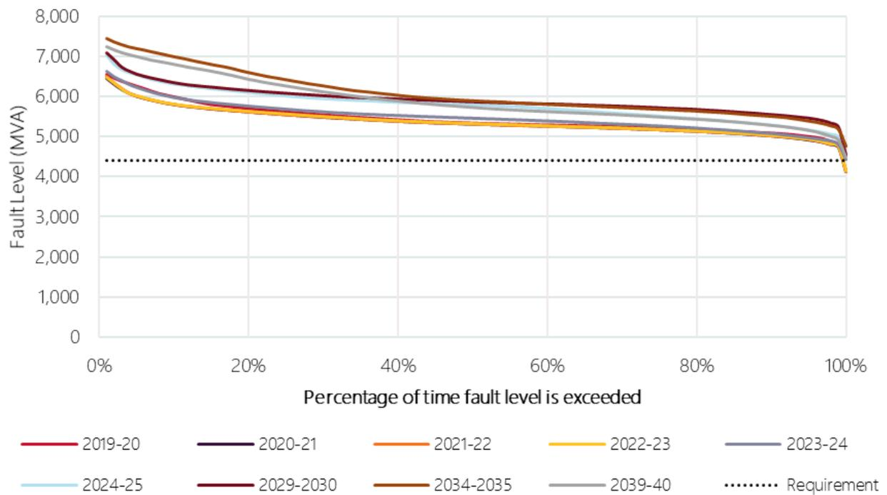
**Figure 177 Projected Dederang 220 kV fault level duration curves**
