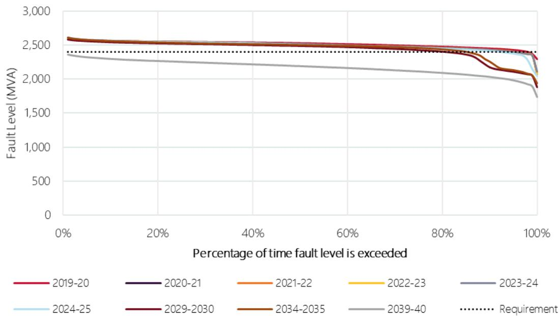
**Figure 162 Projected Lilyvale 132 kV fault level duration curves**
