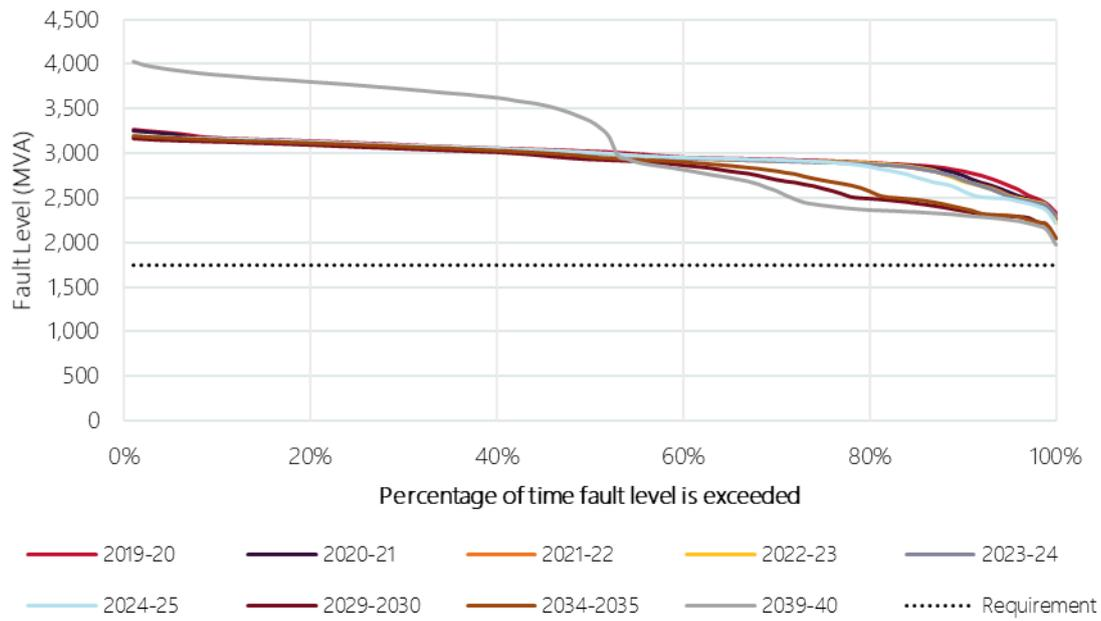
**Figure 161 Projected Gin Gin 275 kV fault level duration curves**
