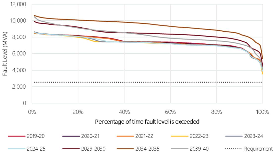
**Figure 159 Projected Greenbank 275 kV fault level duration curves**
