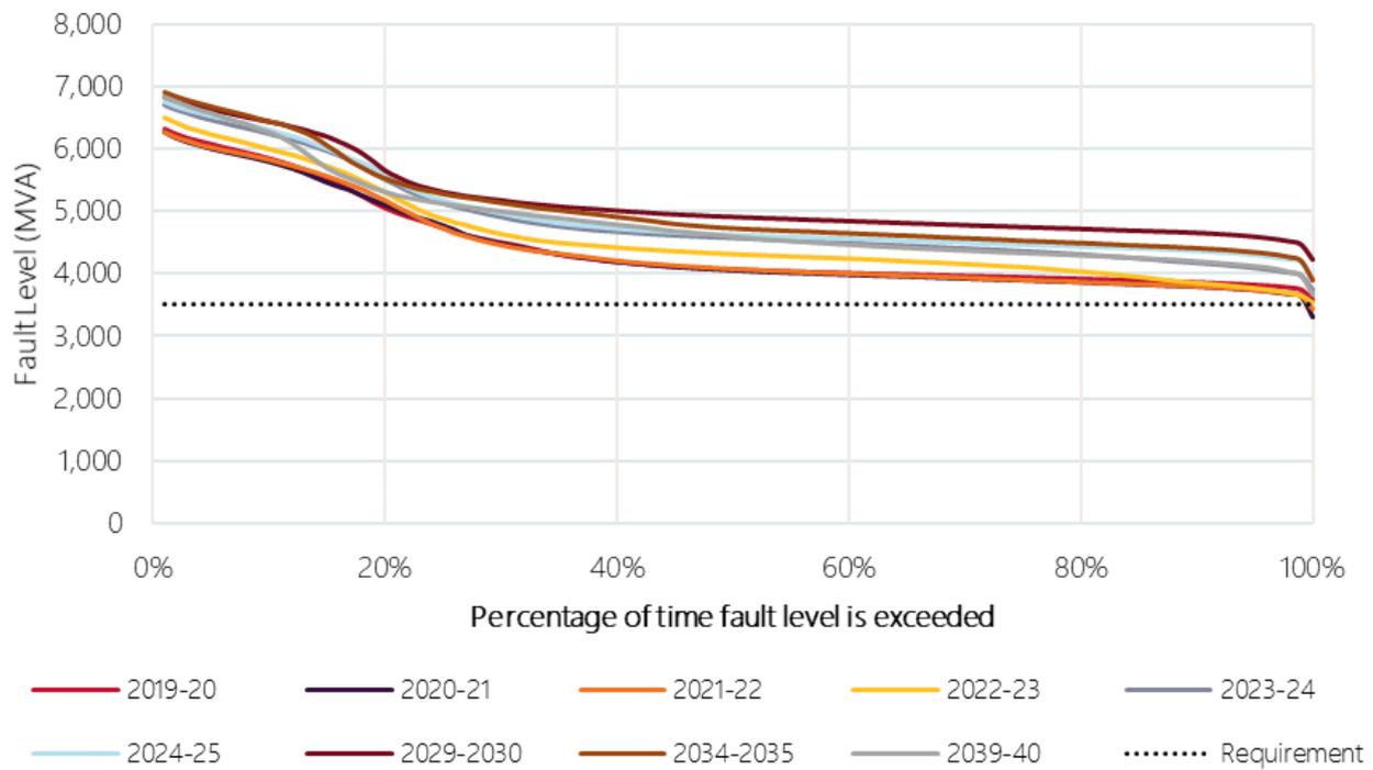
**Figure 178 Projected Hazelwood 500 kV fault level duration curves**
