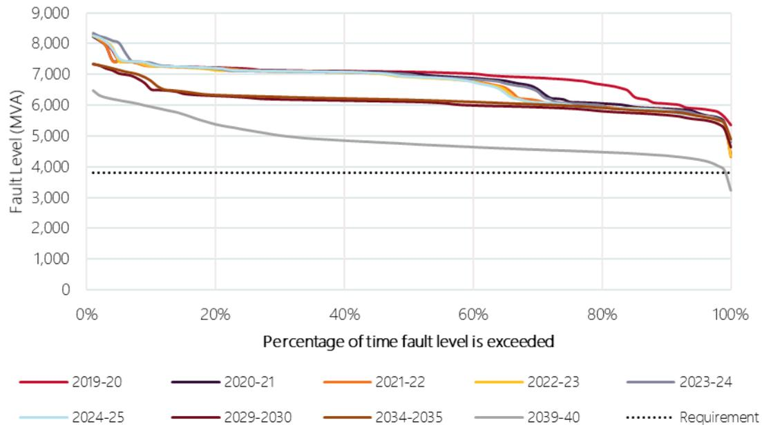
**Figure 160 Projected Nebo 275 kV fault level duration curves**
