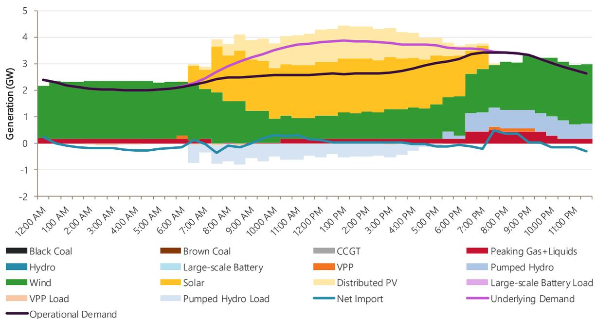
**Figure 73 South Australia – Forecast minimum operational demand 19/02/2040, Central scenario**
