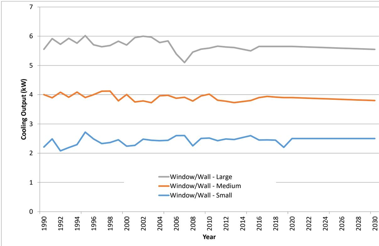
Figure 63: Trends in window wall air conditioner efficiency (EER) by size range to 2030
