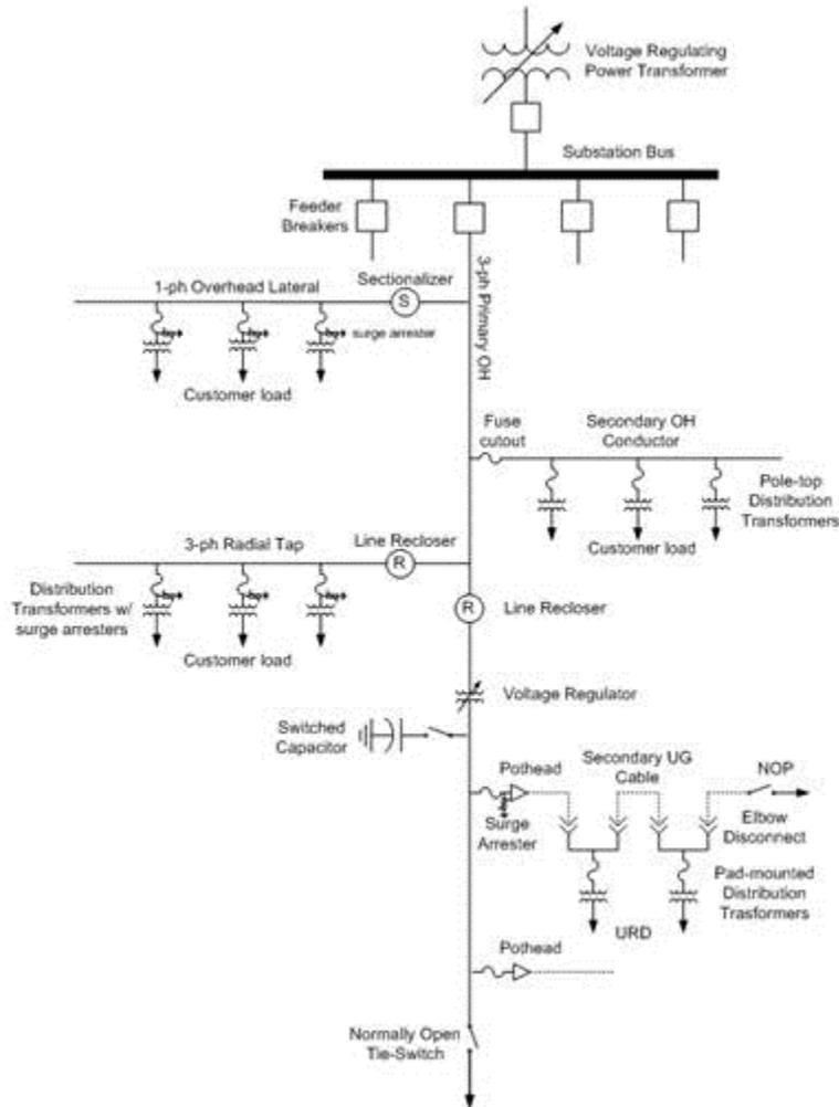
Figure 22 Schematic of a Distribution System
