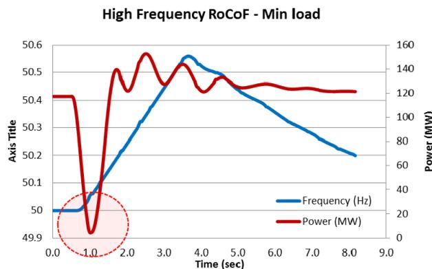
Figure 9 GT response to High RoCoF from Min Load
