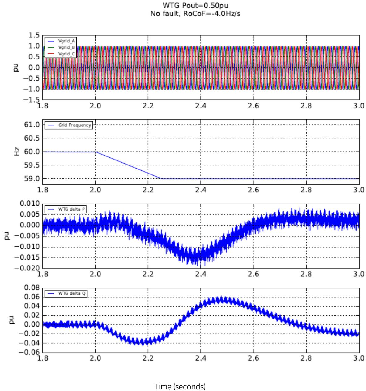
Figure 13 High RoCoF Frequency drop for Type 3 WTG
