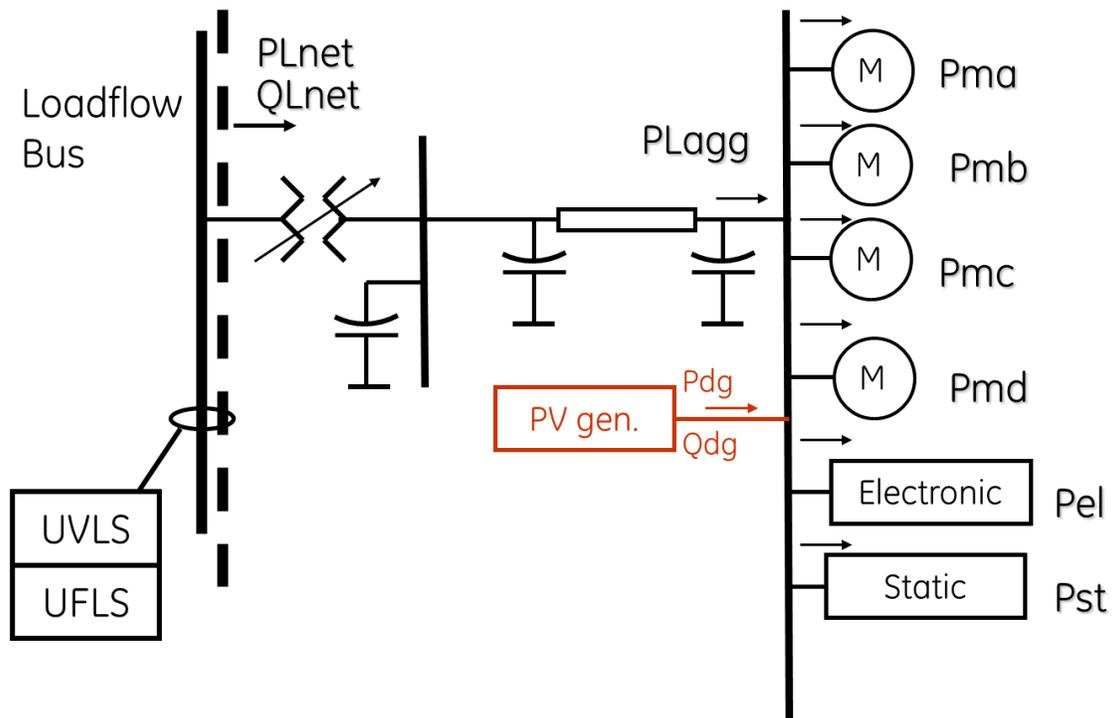
Figure 24 Composite Load Model
