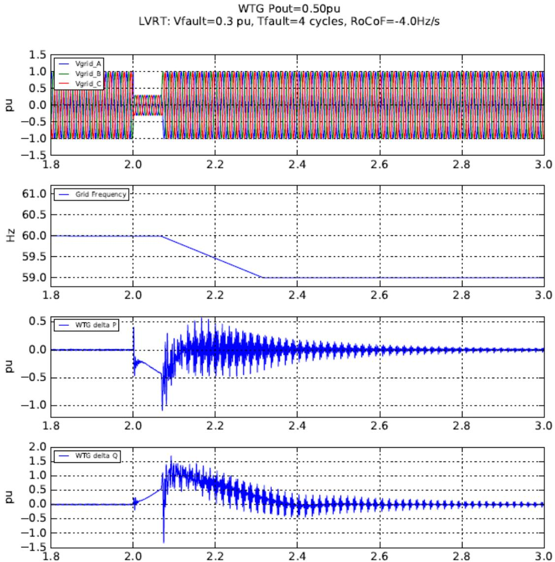
**Figure 18 Response to Grid Fault and High RoCoF decrease for type 4 WTG**
