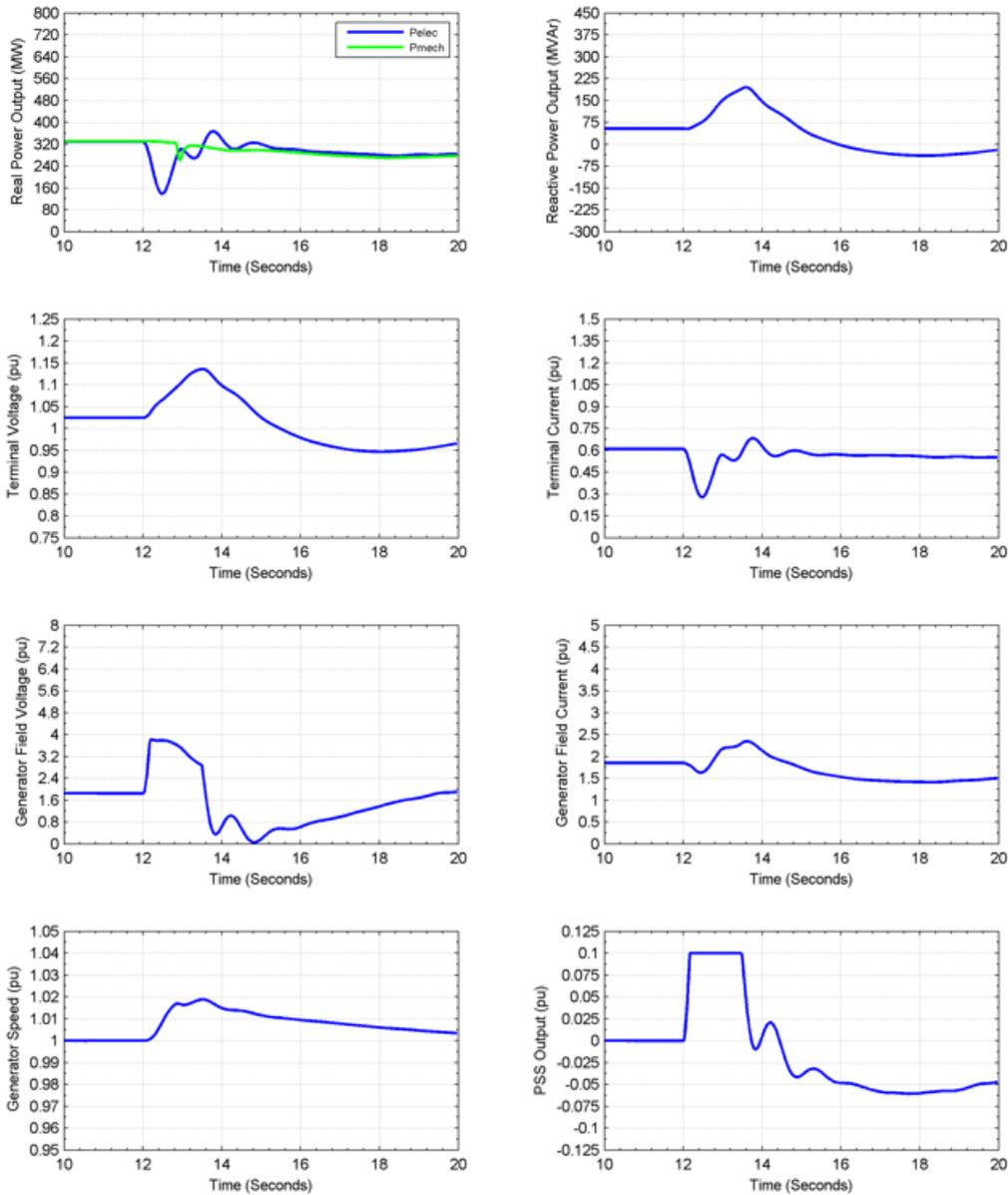
Figure 8 Simulation of 1Hz/sec RoCoF event
