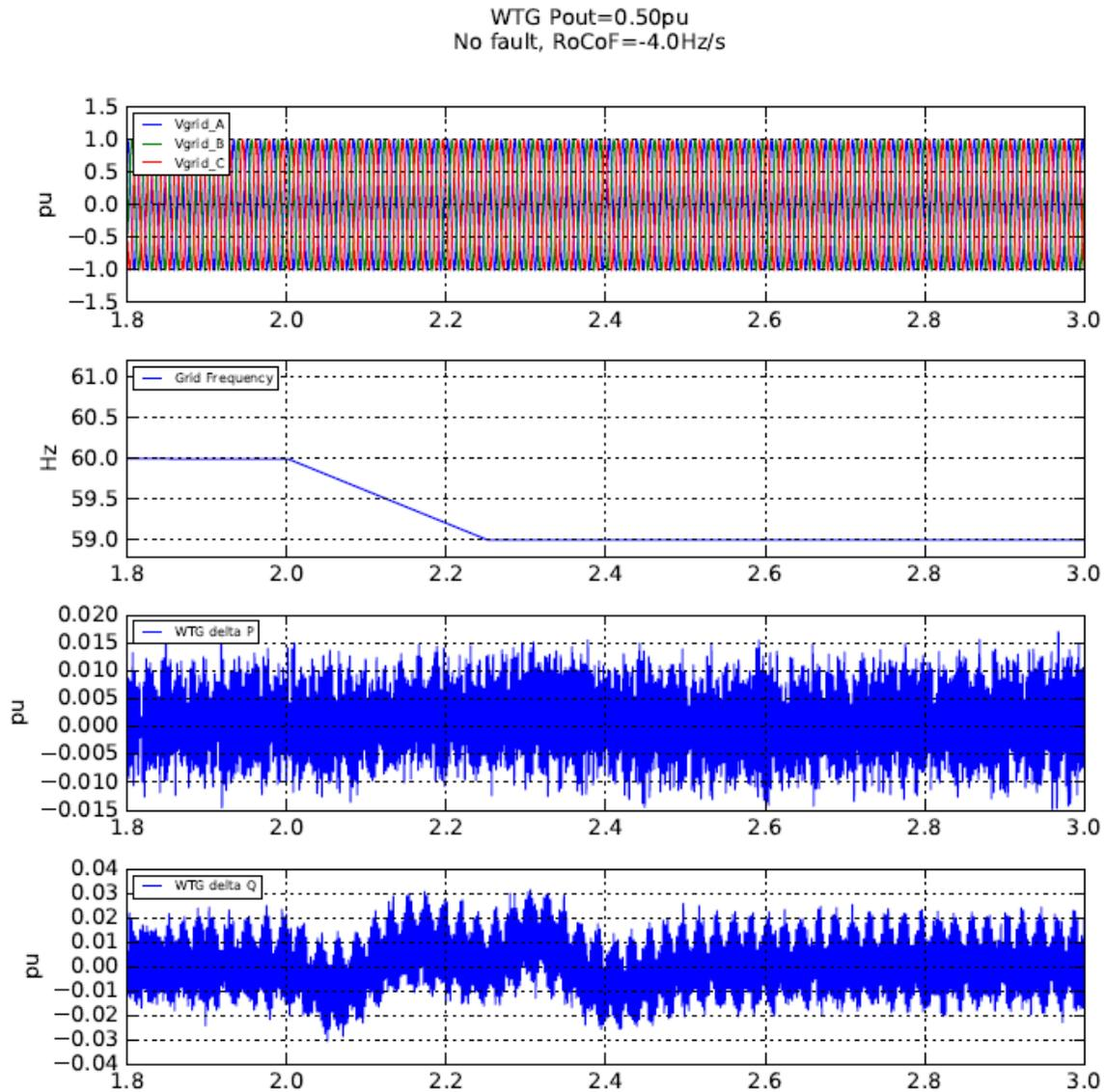
Figure 16 Response of High RoCoF decline for Type 4 WTG
