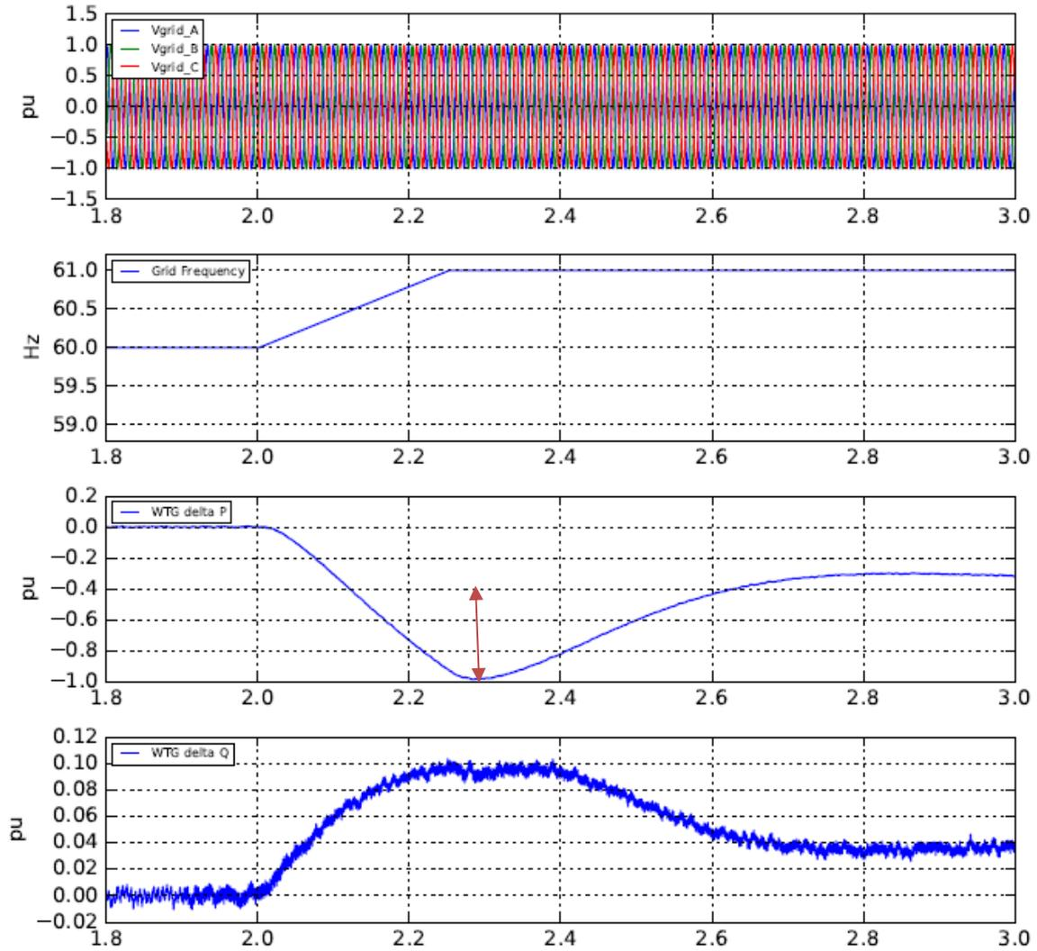
Figure 21 BESS response to high positive RoCoF
