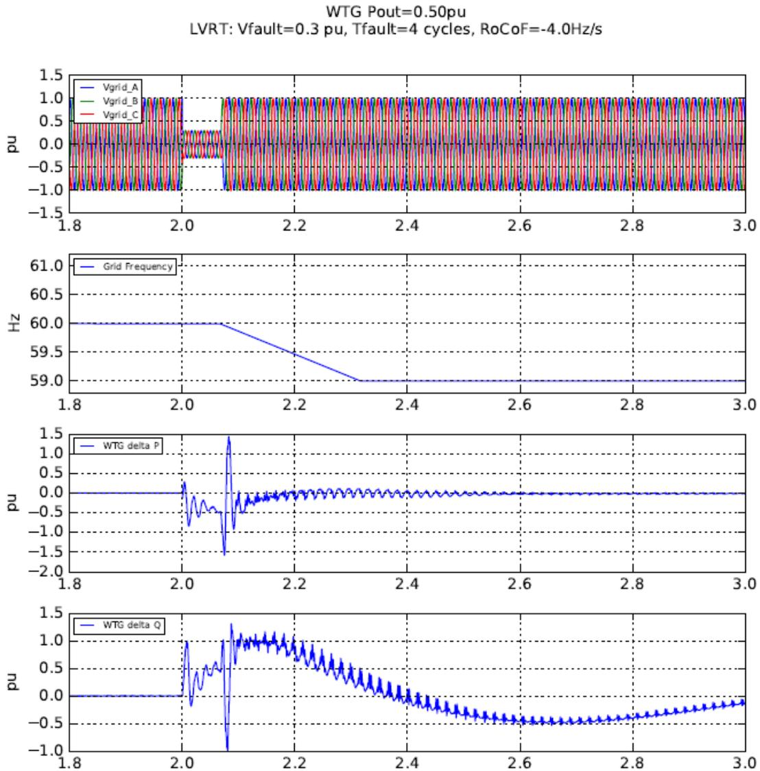
**Figure 15 Grid Fault followed by High RoCoF decline for Type 3 WTG**
