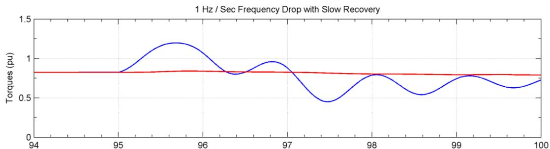
Figure 4 Electrical (Blue) and Mechanical (Red) Torques to a Simulated RoCoF Event
