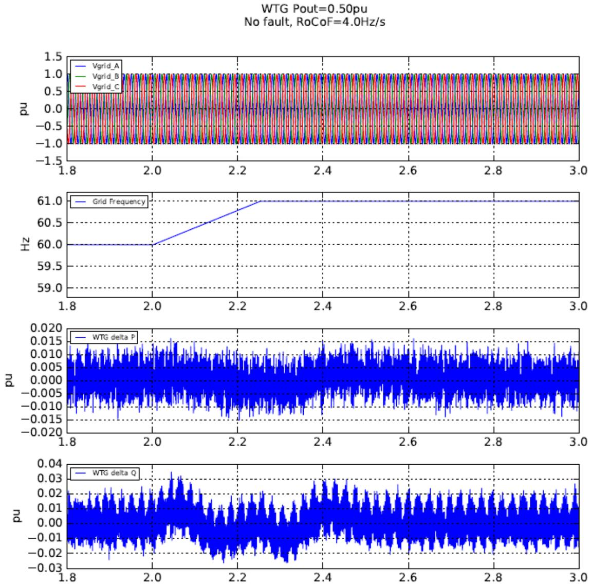
**Figure 17 Response for High RoCoF increase for type 4 WTG**
