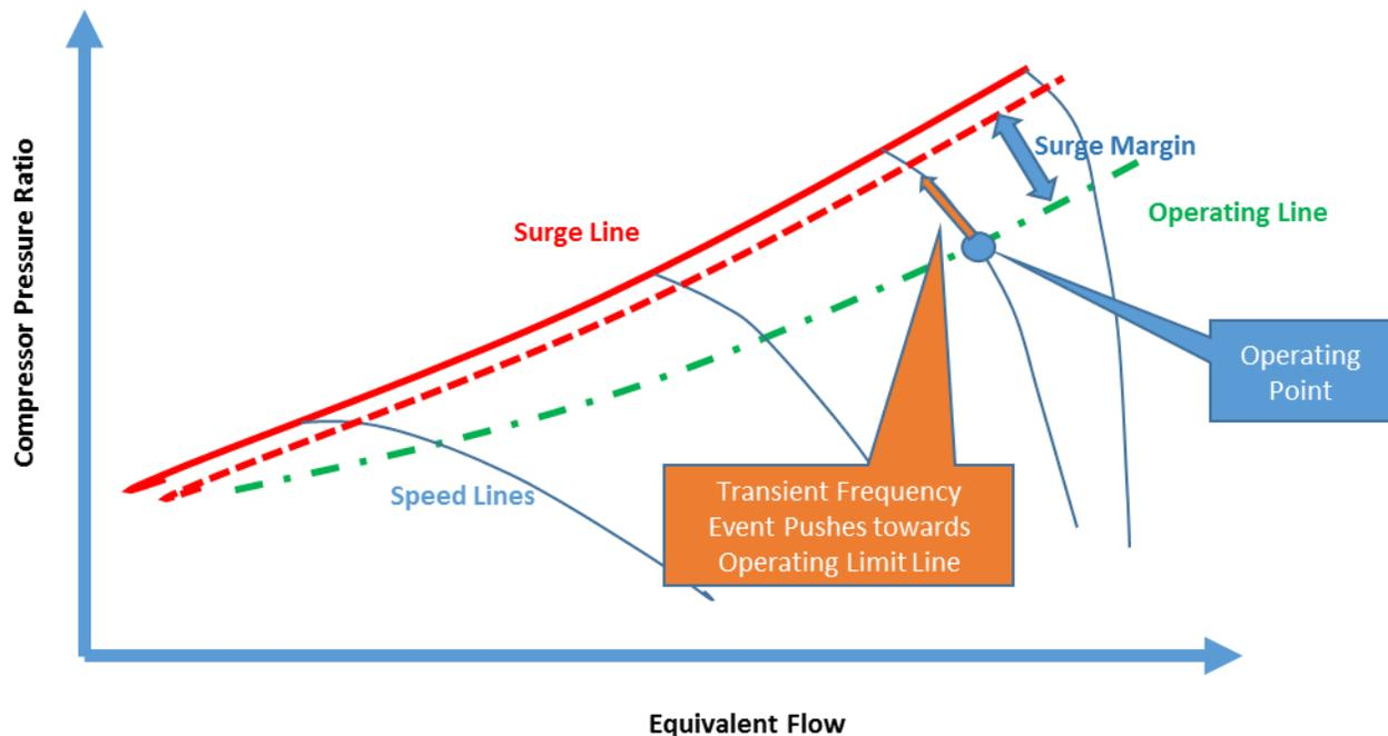
**Figure 3 Generic Compressor Performance Map of an Axial Compressor**
