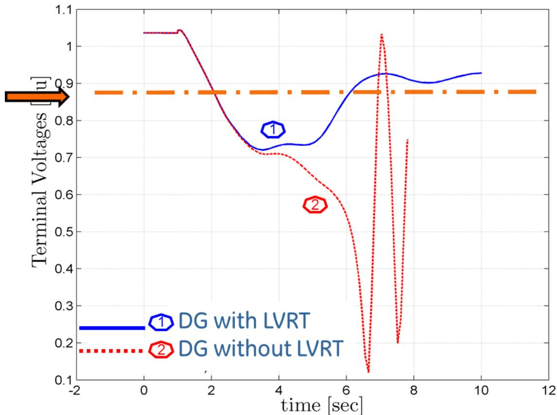
Figure 27 Illustration of Impact of Distributed PV Fault-ride Through on Bulk System
