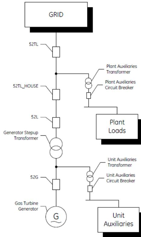
**Figure 5 Synchronous Generation Relay Schematic**
