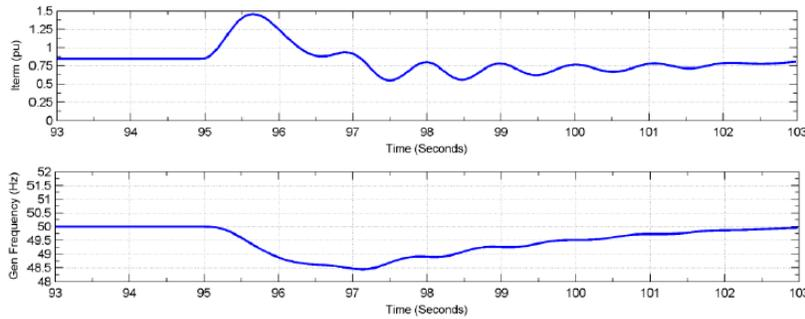
**Figure 10 Over-current Illustration (simulations)**
