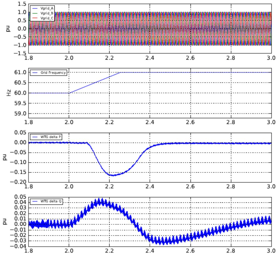
Figure 14 High RoCoF Frequency Rise for Type 3 WTG
