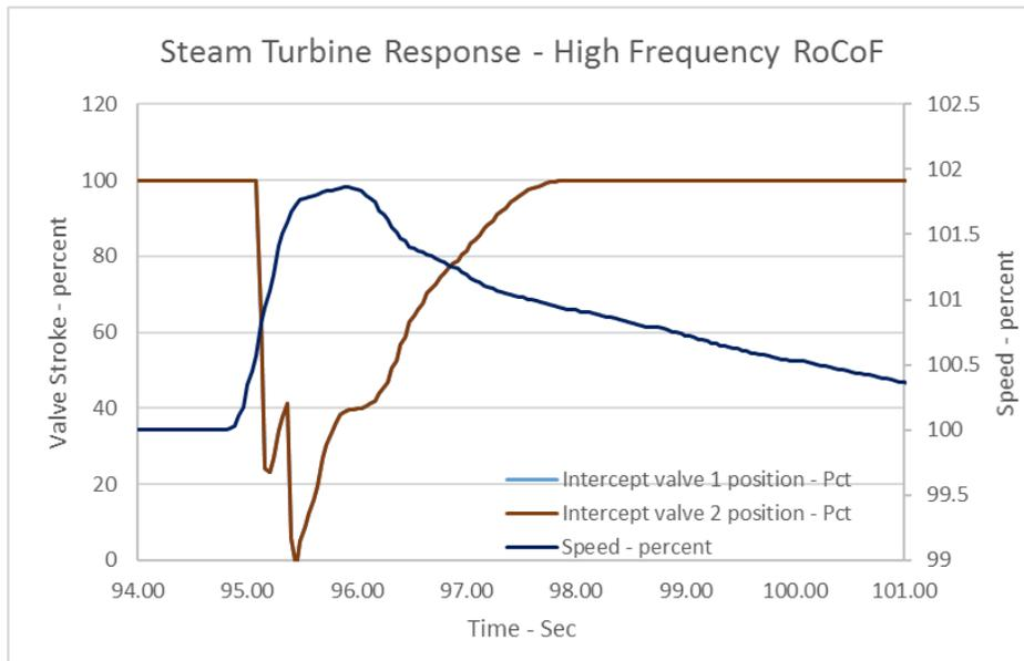
**Figure 7 Measured Response of Steam turbine for RoCoF event**
