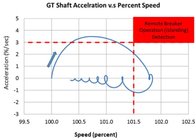
**Figure 6 GT Acceleration Trajectory for Positive RoCoF Event**
