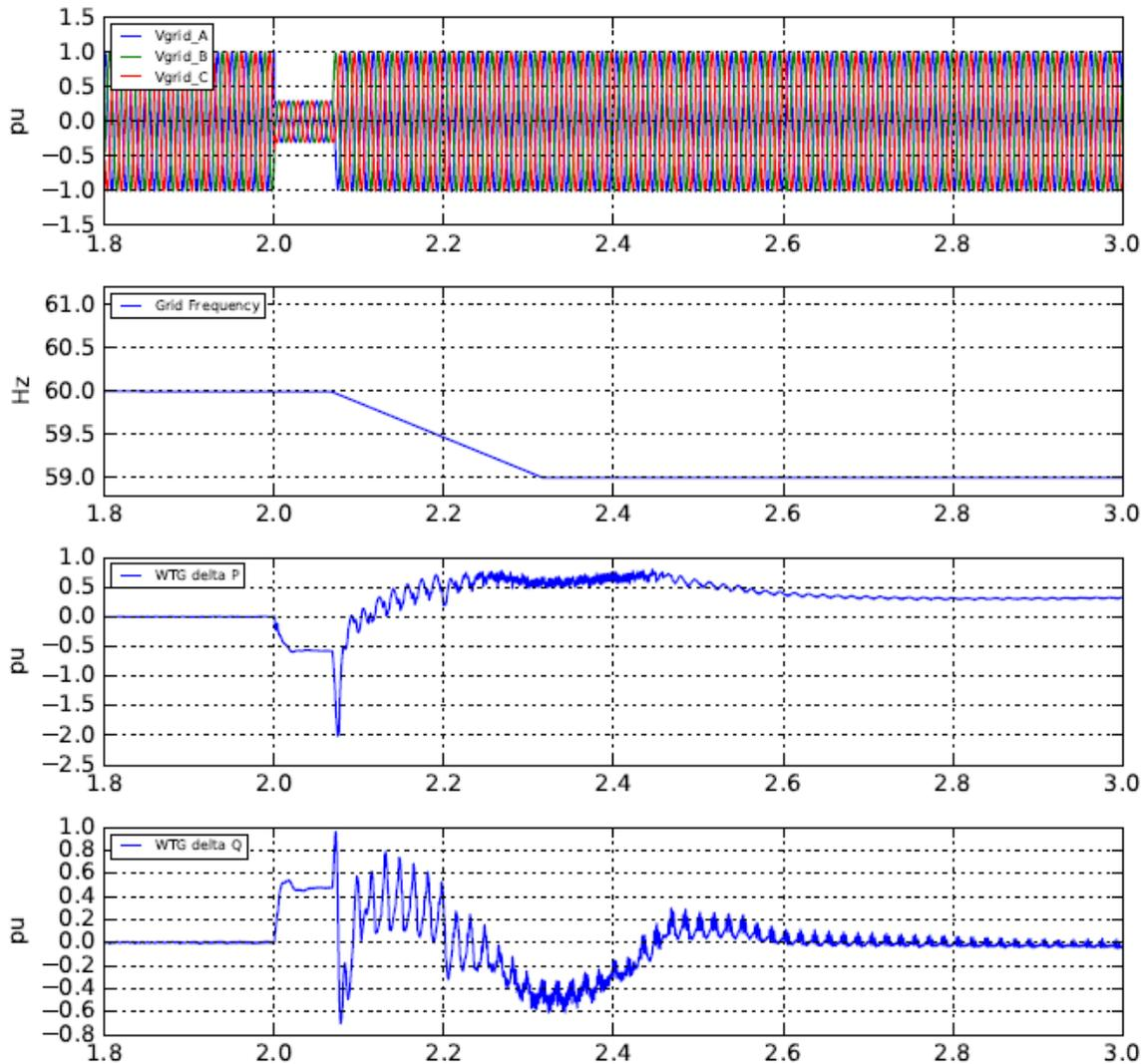
Figure 20 BESS Response to Grid Fault and High RoCoF decrease
