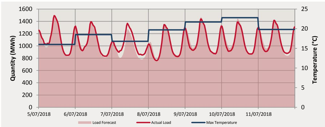
The maximum temperatures for this trading week ranged from 16°C to 22.8°C. The actual load peaked at 1493.099 MWh on the 5/7/2018.
