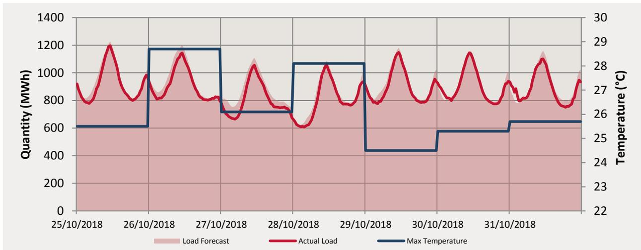
The maximum temperatures for this trading week ranged from 24.5°C to 28.7°C. The actual load peaked at 1196.888 MWh on the 25/10/2018.
