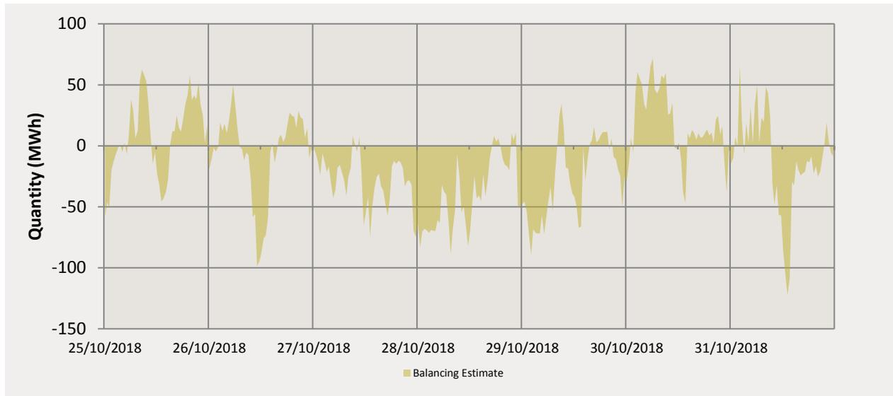
The majority of the balancing activity this week occurred within Balancing Supply. The maximum balancing demand for the week reached 71.7295 MWh on the 30/10/2018. The maximum balancing supply for the week reached -122.377 MWh on the 31/10/2018.
