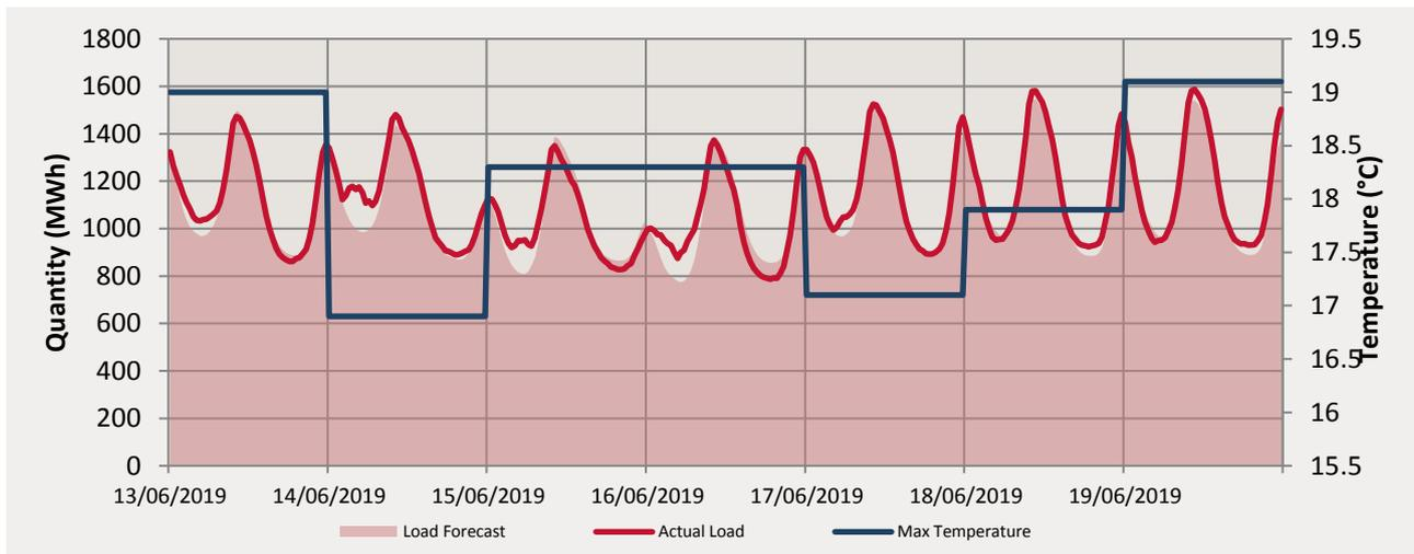
The maximum temperatures for this trading week ranged from 16.9°C to 19.1°C. The actual load peaked at 1586.983 MWh on the 19/6/2019.
