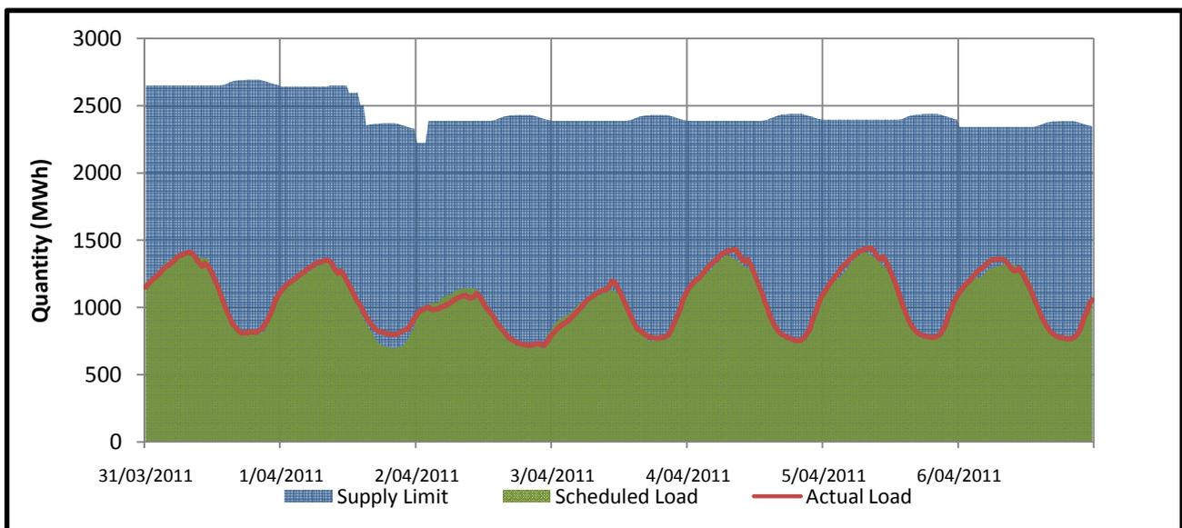
The supply limit ranged from 2225.407 MWh to 2694.271 MWh with the Scheduled System Load peaking at 1416.553 MWh on the 5/4/2011.
