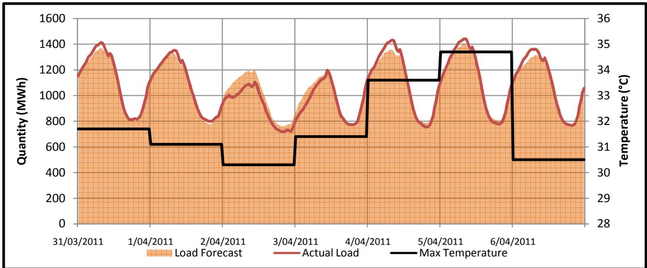
The maximum temperatures for this trading week ranged from 30.3°C to 34.7°C. The actual load peaked at 1441.338 MWh on the 5/4/2011.
