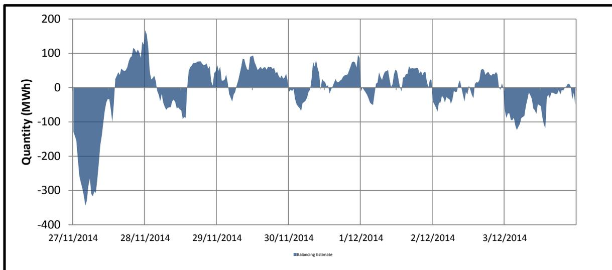
The majority of the balancing activity this week occurred within Balancing Supply. The maximum balancing demand for the week reached 167.1525 MWh on the 28/11/2014. The maximum balancing supply for the week reached -343.956 MWh on the 27/11/2014.
