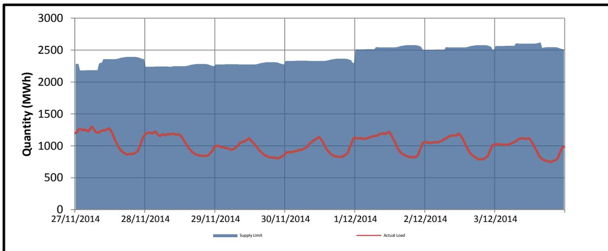
The supply limit ranged from 2181.379 MWh to 2622.159 MWh
