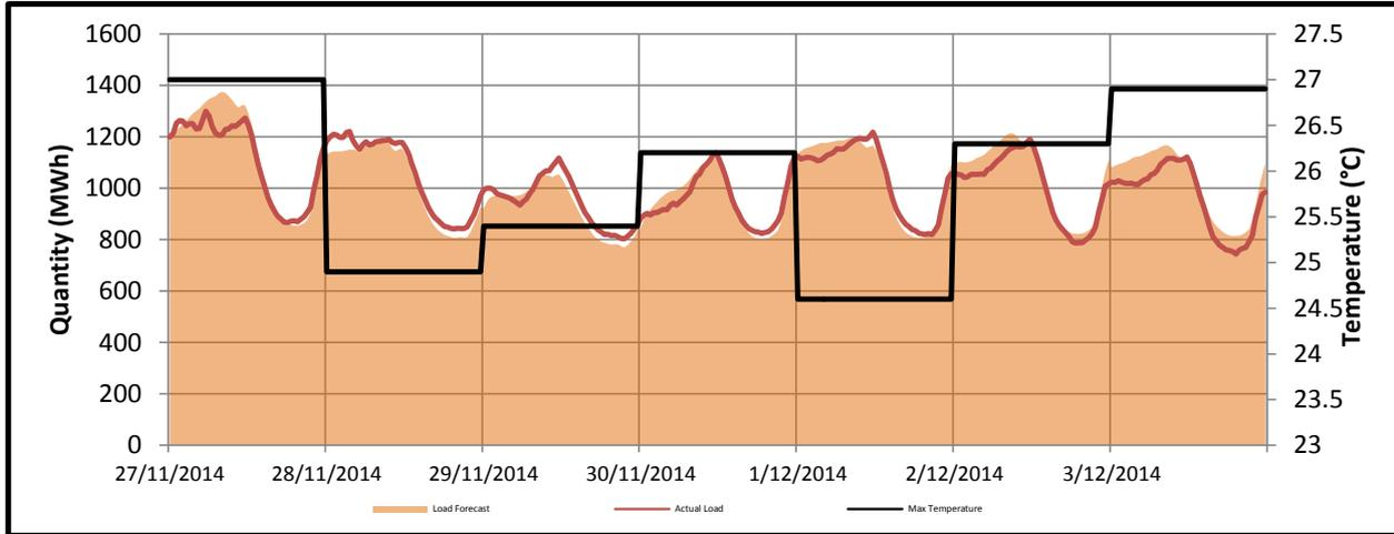
The maximum temperatures for this trading week ranged from 24.6°C to 27°C. The actual load peaked at 1299.55 MWh on the 27/11/2014.
