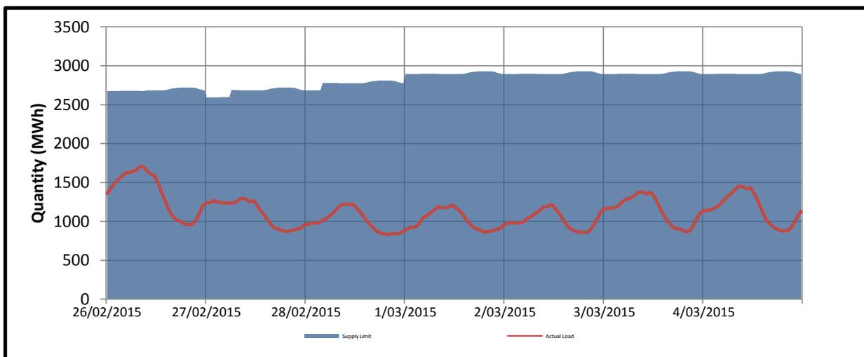
The supply limit ranged from 2594.533 MWh to 2929.316 MWh
