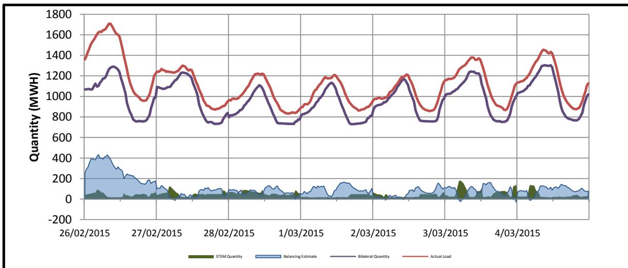
Total balancing supply equalled -119.581 MWh whereas total balancing demand equalled 35471.294 MWh. The Total STEM Traded quantity was 15426.906 MWh, with the STEM Clearing Quantity ranging between 13.91 MWh and 180.139 MWh.
