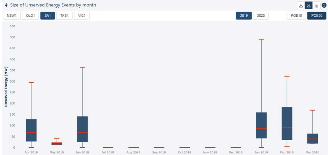
Figure 10: Size of Unserved Energy events by month (User to select POE Demand Level, Region and Year)
