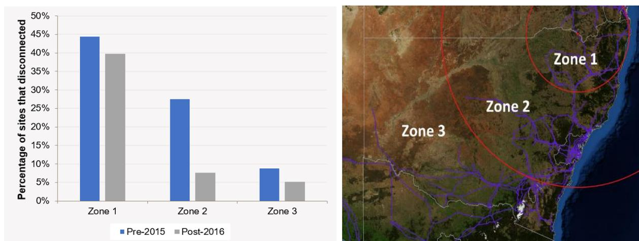
This geographic distribution of reduced generation also reinforces that incrementally improving voltage disturbance withstand capabilities for DER will reduce the amount of DER lost during disturbances. The severity of the voltage dip experienced by DER systems reduces at more distant locations, so incrementally improving their ability to remain operational, limits the impact of a fault to a smaller zone. This will become increasingly important as DER levels grow.
