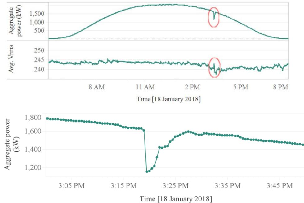
Upscaling to the quantity of distributed PV operating at the time of the event suggests at least 120 MW of distributed PV was lost across Victoria<sup>25</sup>. This likely partially offset the demand reduction that was observed.
