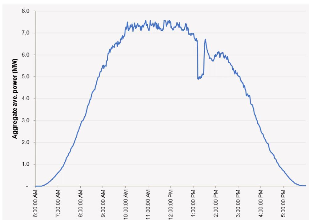
Upscaling the data from the Solar Analytics sample, in tranches by installation date and system size, indicates that generation from distributed PV in Queensland suddenly reduced by approximately 165 MW (17%) at the time of the event.
