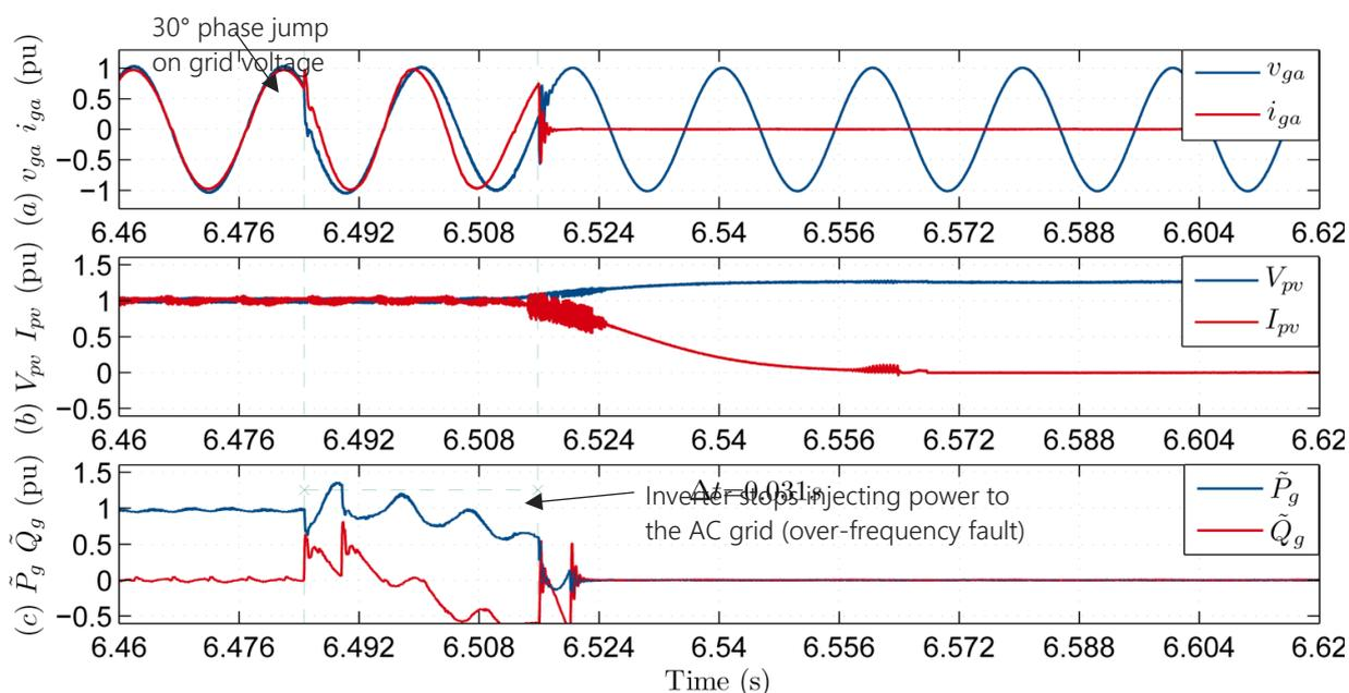
Note: The y-axis in order are Chart (a) Blue: Grid Voltage(100V/div), Red: Grid Current (10A/div), Chart (b) Blue: Inverter Voltage (200V/div), Red: Inverter Current (5A/div), Chart (c) Blue: Inverter Real power injection to the Grid, Red: Inverter Reactive power to the grid. The x-axis time base is 10 ms/div.
