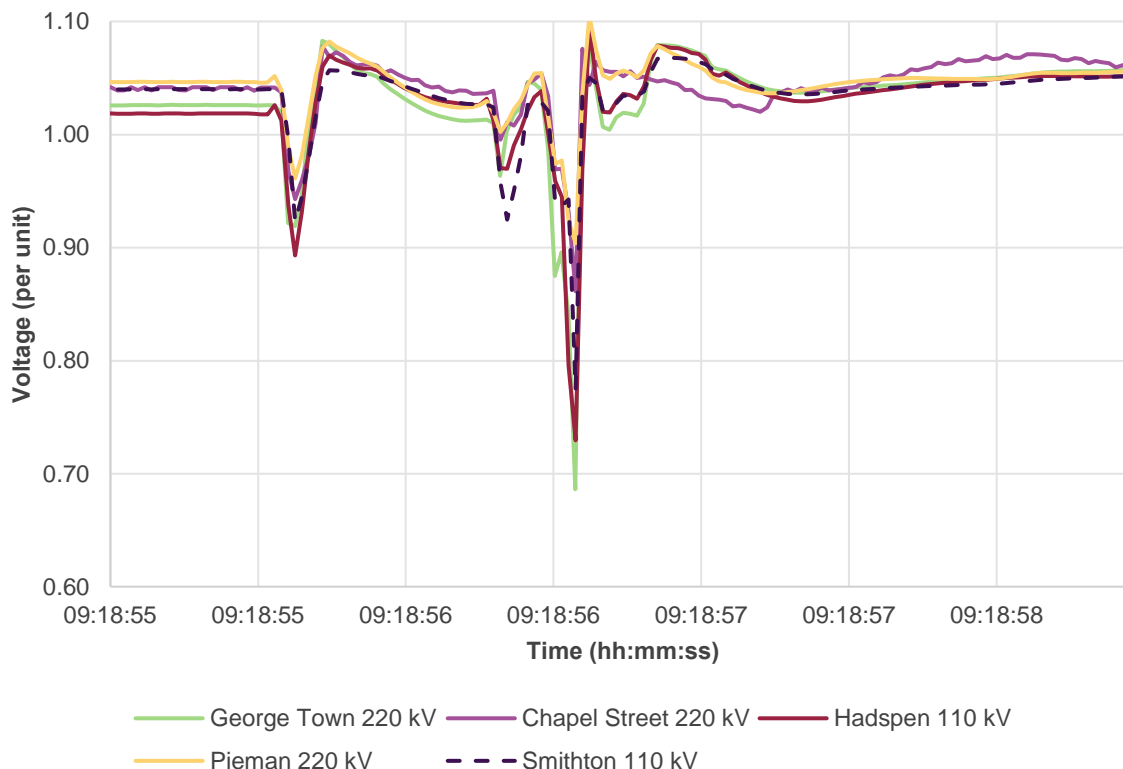
Figure 4 Voltages during incident (PMU) zoomed in on initial voltage disturbances
