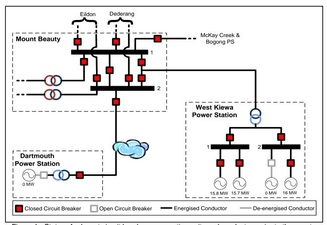
Figure 1 - Status of relevant circuit breakers, generating units and conductors prior to the event
