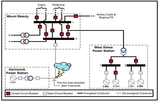
Figure 2 - Status of relevant circuit breakers, generating units and conductors immediately after the event
