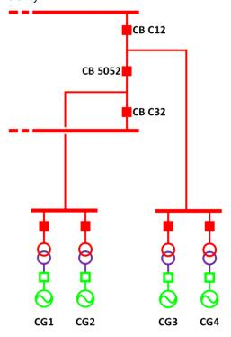
System configuration immediately after the incident. Elements not related to this incident have been omitted for clarity.
