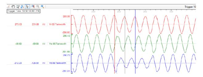
The figures below show the neutral current in the 85 line and the 86 line as measured at Armidale at the time of the fault on the 96C line.
