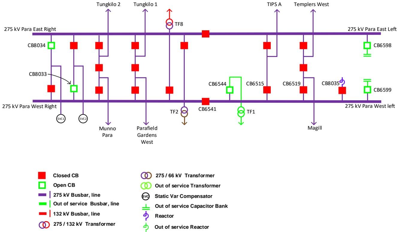
Figure 2 Incident diagram – Para substation equipment status immediately following the incident
