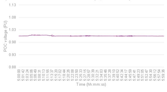
Figure 11 Murra Warra Wind Farm POC measured single phase RMS voltage
