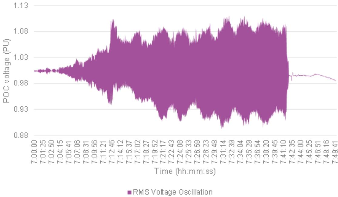
**Figure 11** Murra Warra Wind Farm POC measured single phase RMS voltage
