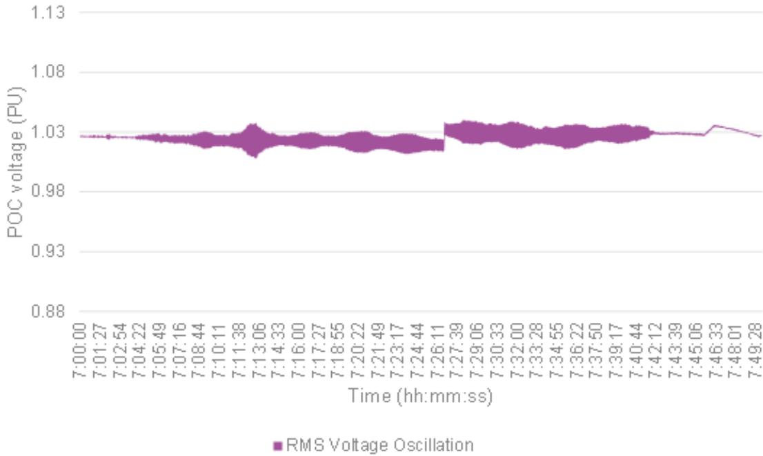
**Figure 9** Wemen Solar Farm POC measured single phase RMS voltage
