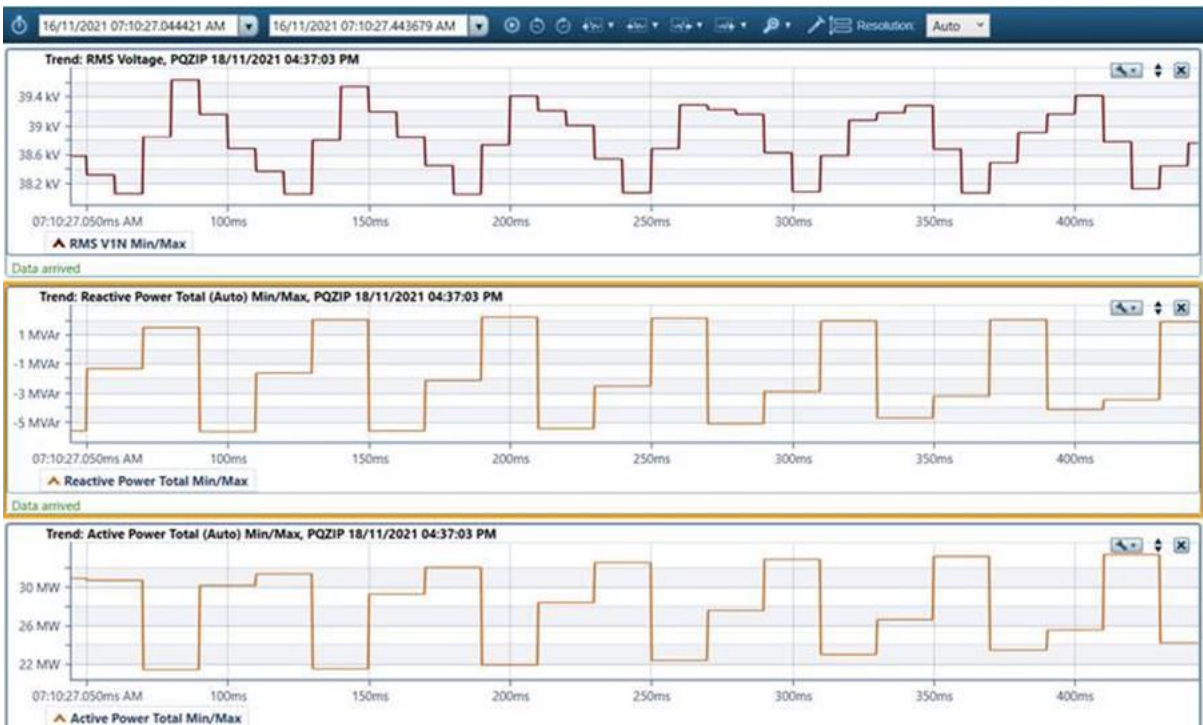
Figure 19 Wemen Solar Farm, 0610 hrs on 16 November 2021, Q and V (both in-phase and out-of-phase)
