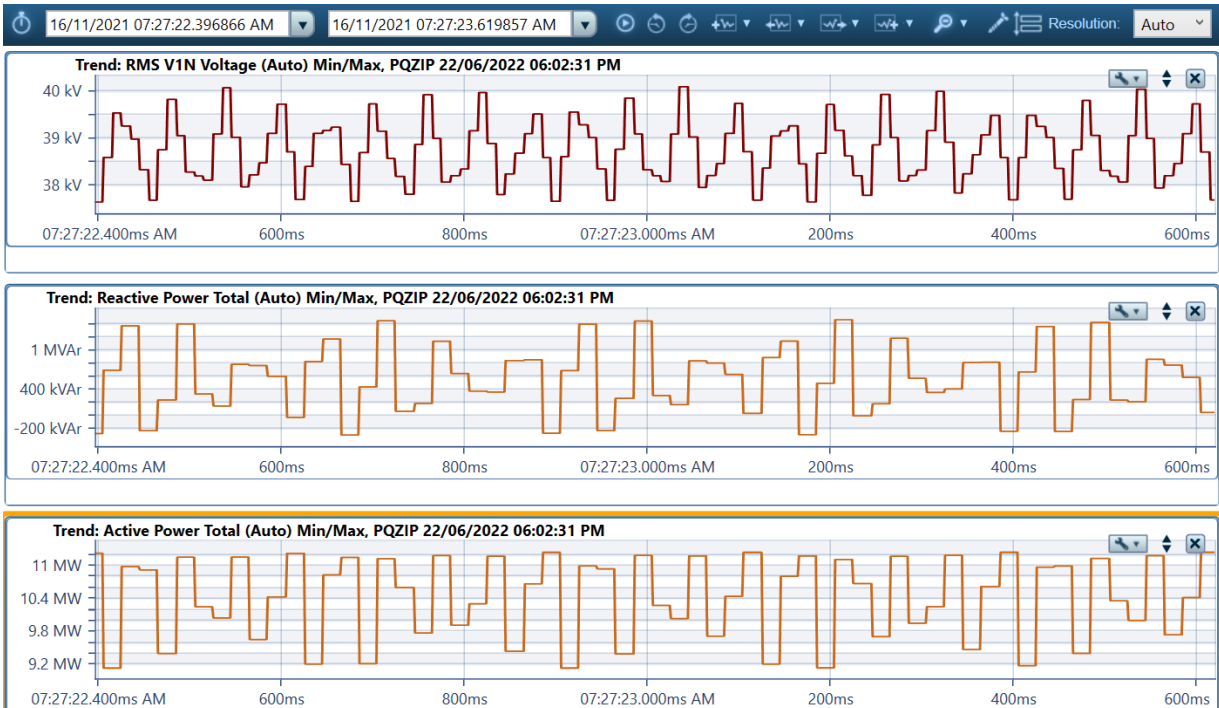
Figure 21 Wemen Solar Farm, 0627 hrs on 16 November 2021, Q and V (both in-phase and out-of-phase)
