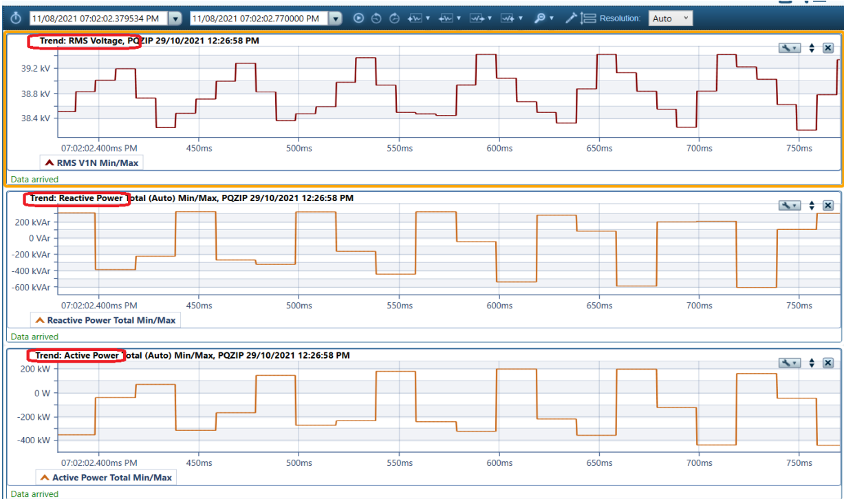
Figure 15 Bannerton Solar Farm, 11 August 2021 event, Q and V relation in and out of phase
