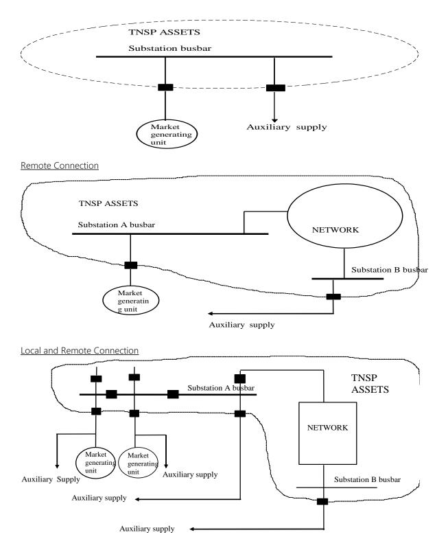
In all cases above, auxiliary supply for the *market generating unit* is taken from physically separated *connection points*, either at the same substation, or another point in the *network*, or a combination of local and remote points.
