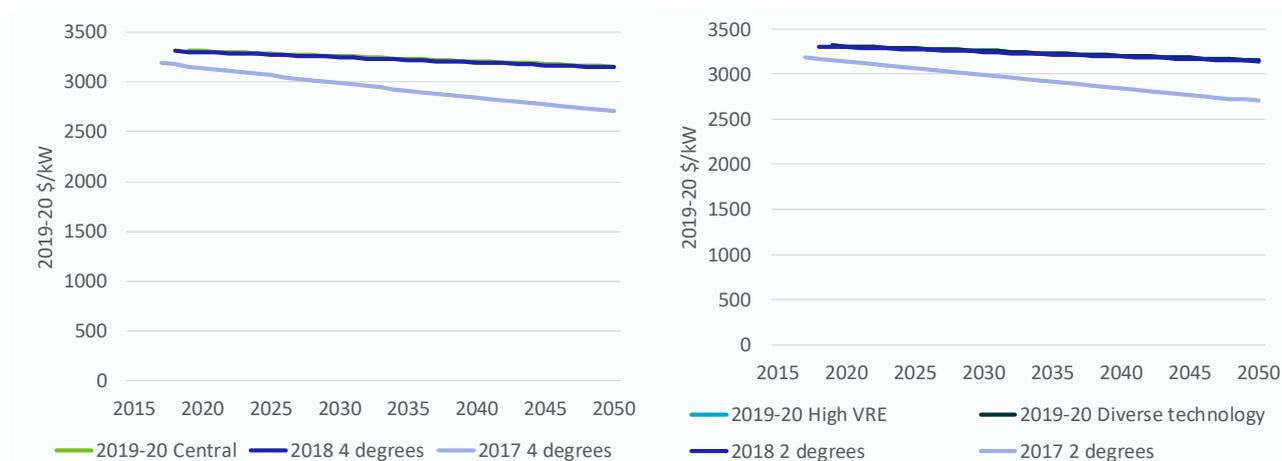
Figure 3-2 Projected capital costs for black coal supercritical by scenario compared to two previous studies
