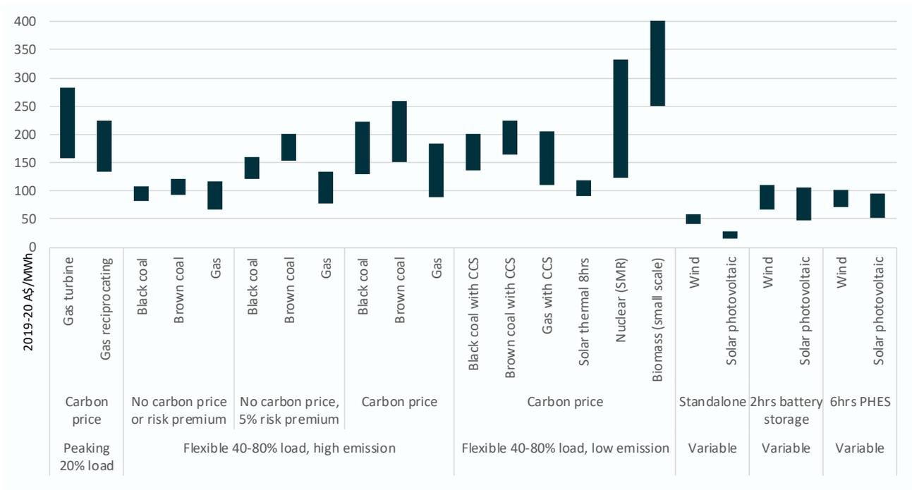
Figure 4-4 Calculated LCOE by technology and category for 2050
