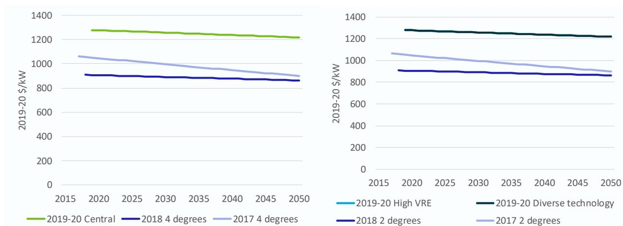
Figure 3-7 Projected capital costs for gas open cycle by scenario compared to two previous studies
