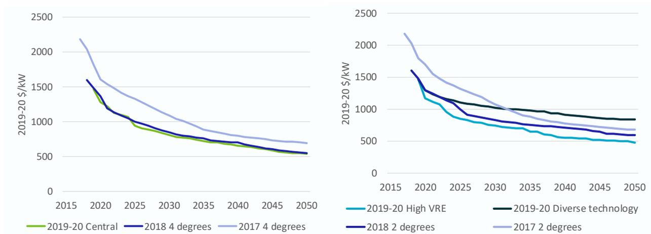
Figure 3-10 Projected capital costs for large scale solar PV by scenario compared to two previous studies
