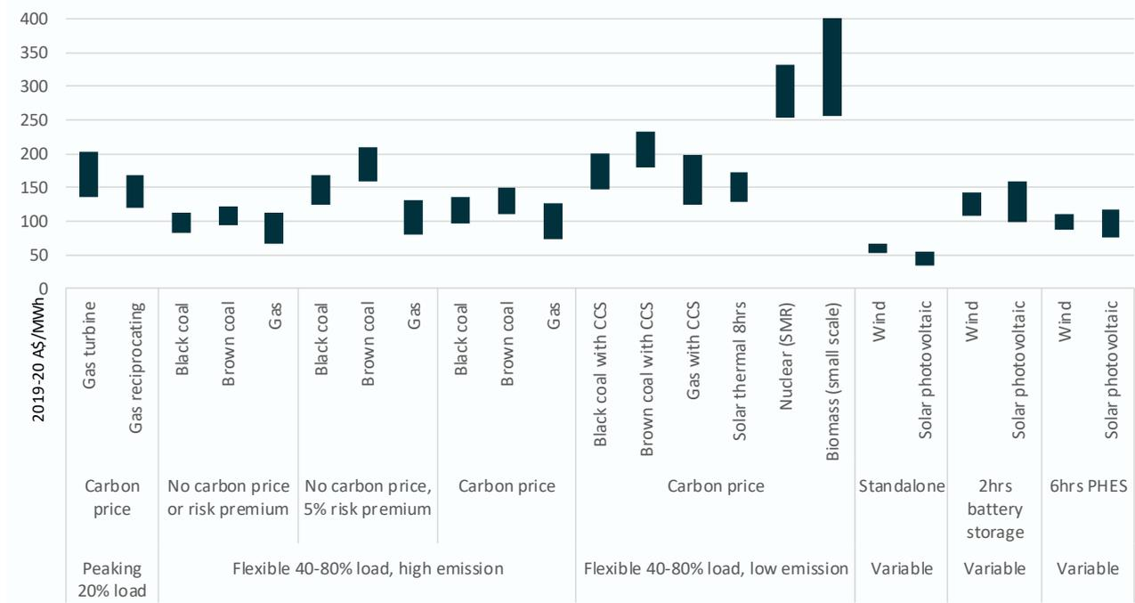
Figure 4-1 Calculated LCOE by technology and category for 2020
