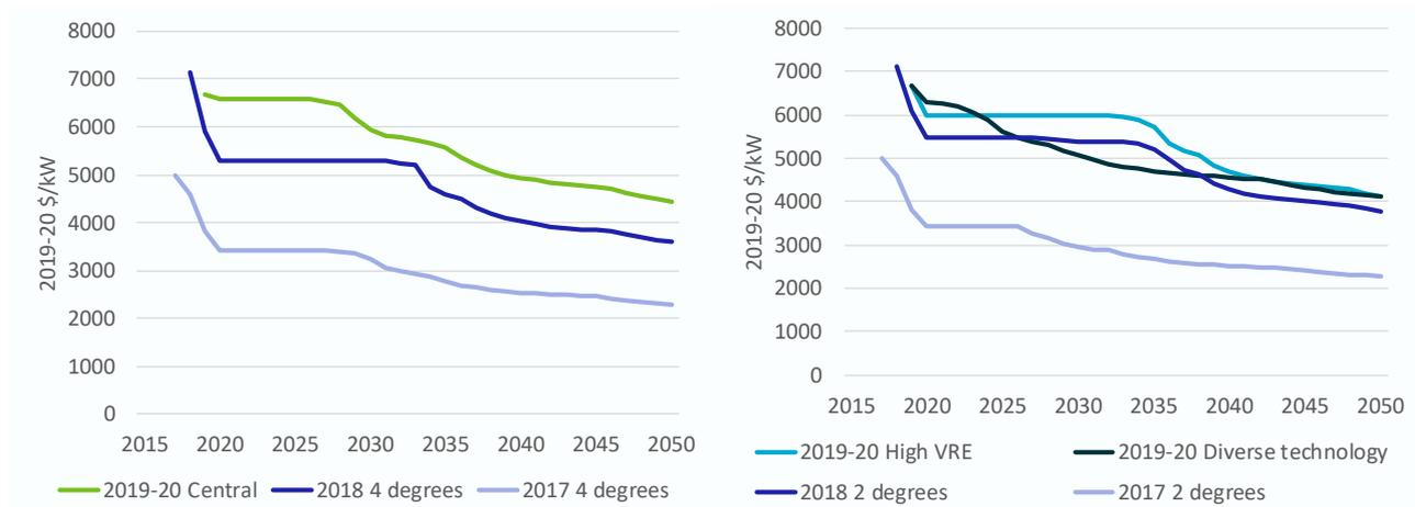
Figure 3-9 Projected capital costs for solar thermal with 8 hours storage by scenario compared to two previous studies
