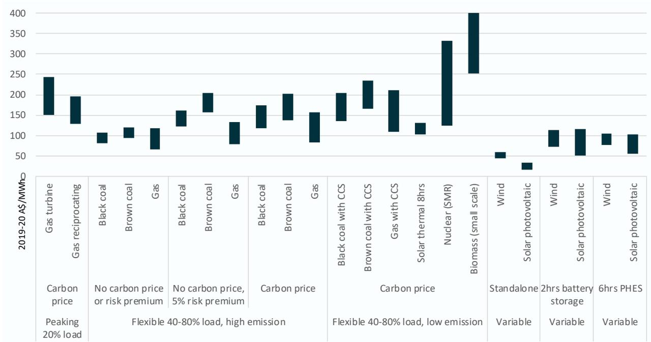
Figure 4-3 Calculated LCOE by technology and category for 2040
