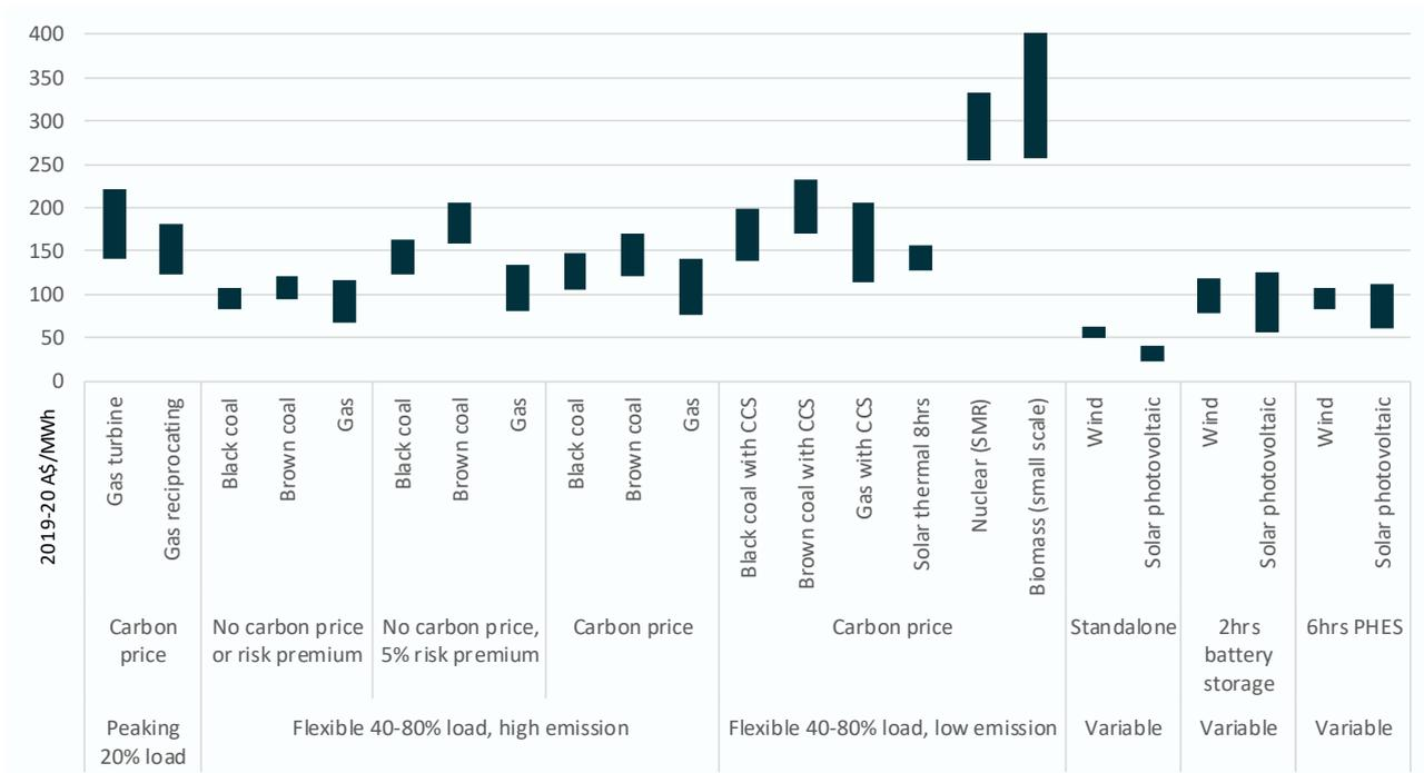
Figure 4-2 Calculated LCOE by technology and category for 2030
