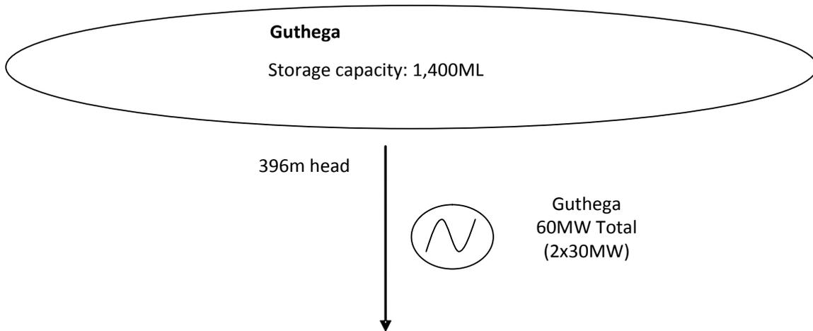
Figure 16 Shoalhaven power station hydro model
