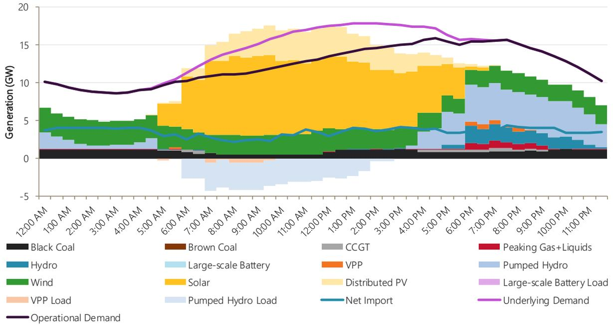
**Figure 69 New South Wales – forecast minimum operational demand 01/04/2040, Central scenario**
