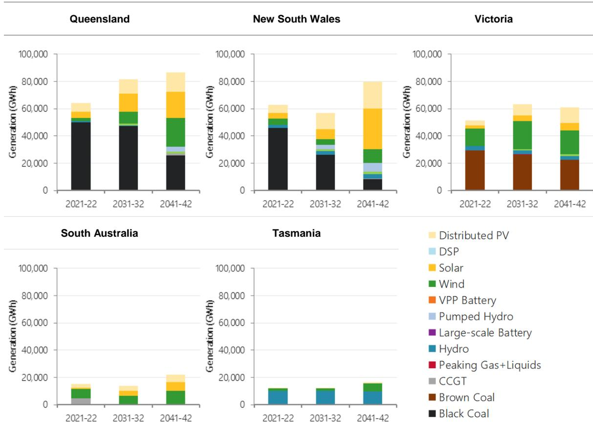
Figure 16 shows the forecast VRE diversity across the NEM. Given the scale of DER developments, this scenario represents reduced diversity of large-scale generation, although the nature of DER is that it will be naturally diversified, with distribution across each region’s population centres.
