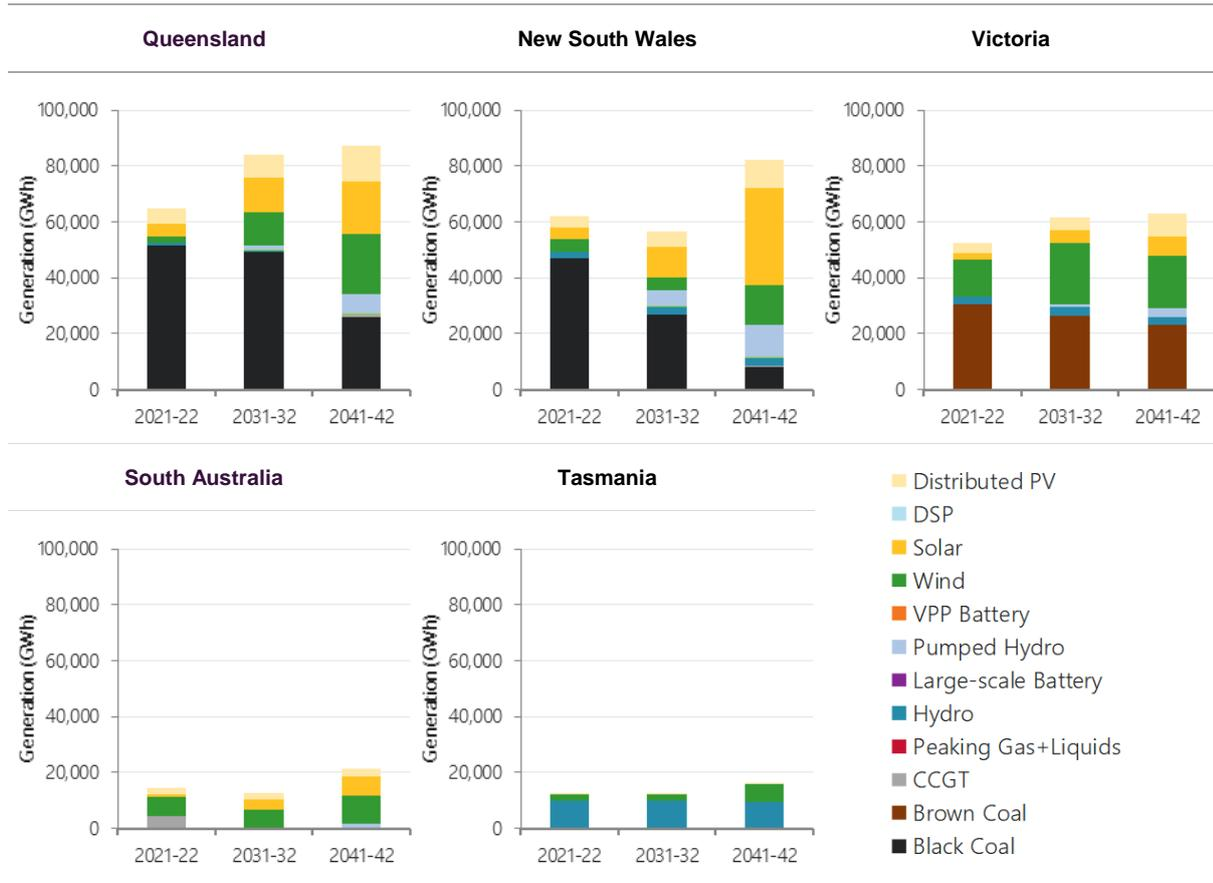
Figure 8 shows the forecast diversity of renewable generation across the NEM, including existing and committed capacity. Geographic and technical diversity will be important to maximise resilience and fuel security associated with weather events, and bushfire risks in a future energy system with high VRE.
