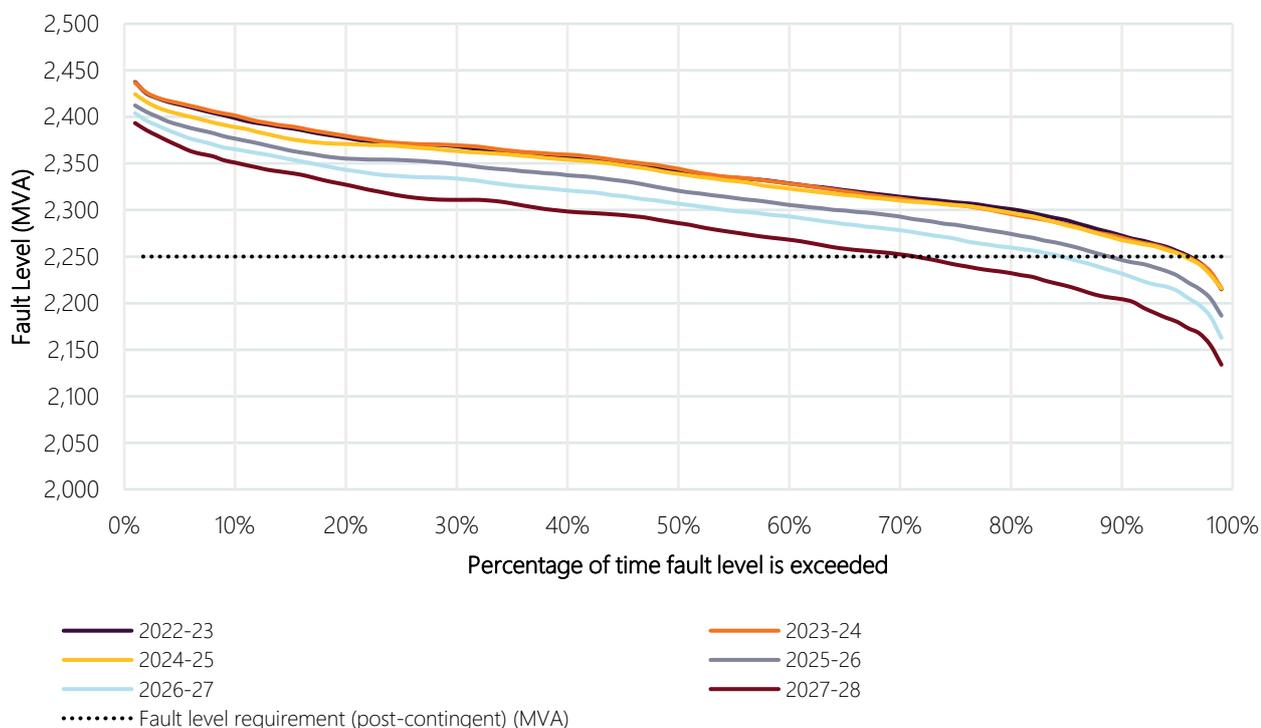
**Figure 18 Greenbank node fault level duration curve against the minimum fault level requirement**
