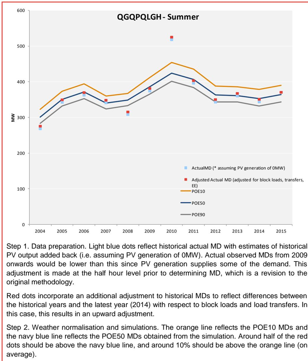
Step 1. Data preparation. Light blue dots reflect historical actual MD with estimates of historical PV output added back (i.e. assuming PV generation of 0MW). Actual observed MDs from 2009 onwards would be lower than this since PV generation supplies some of the demand. This adjustment is made at the half hour level prior to determining MD, which is a revision to the original methodology.
