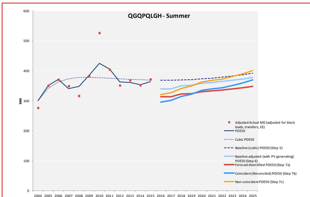
Step 5. The **navy blue dashed line** shows the Baseline forecasts, which reflect the starting point and trend for the cubic trend line (selected in the previous step).
