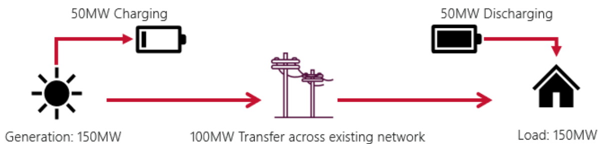
Figure 45 Conceptual representation of virtual transmission line
