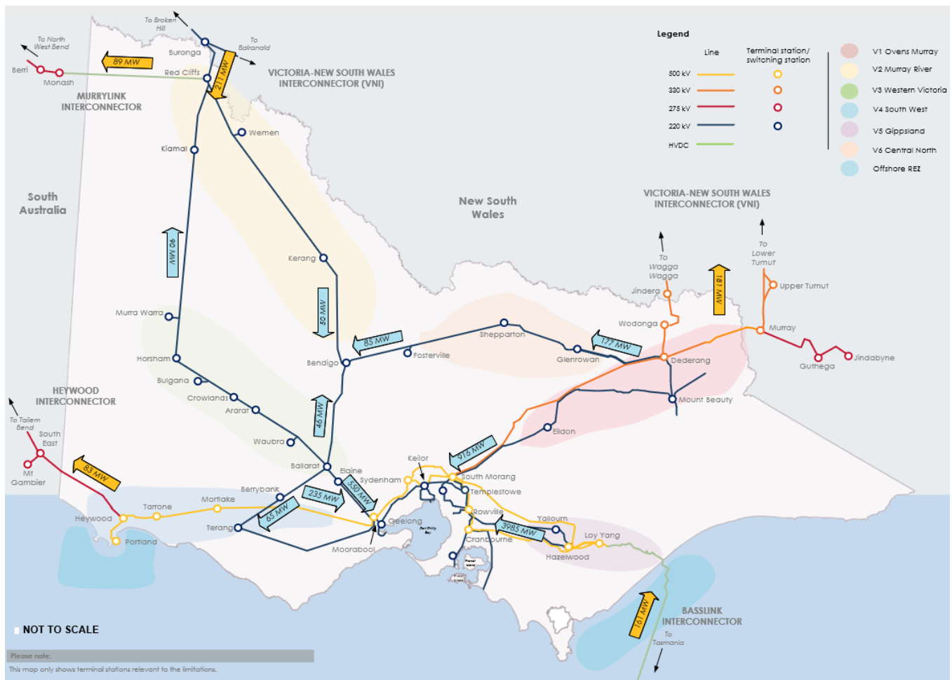
Figure 17 Map of power flows along significant corridors during maximum demand (18:00 on 17 January 2023)
