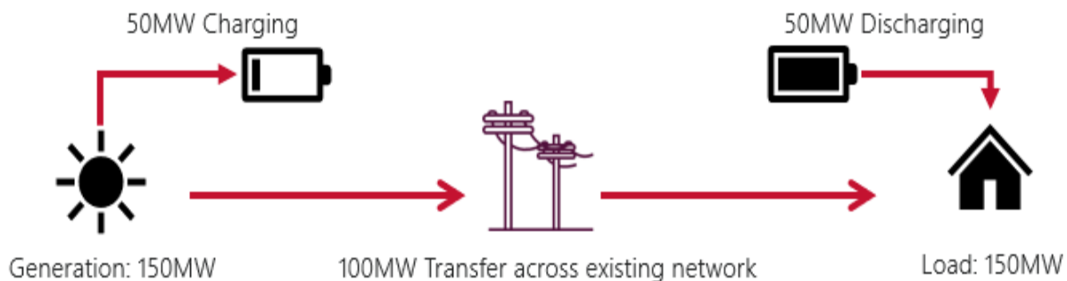
Figure 29 Conceptual representation of virtual transmission line
