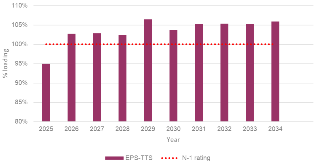
Figure 24 Possible overloading of Eildon – Thomastown 220 kV line under contingencies
