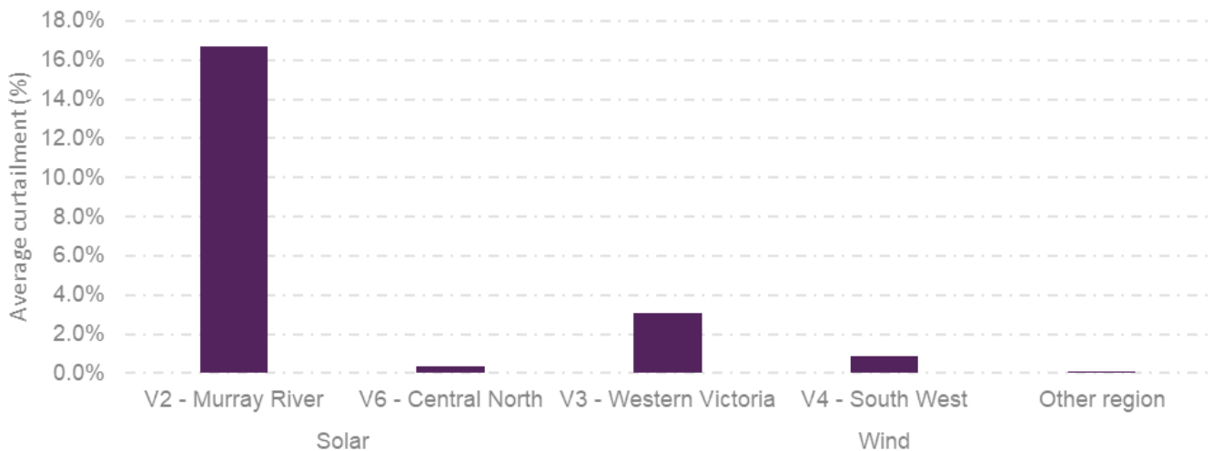
Figure 13 Average VRE network curtailment (%) in Victorian REZs for 2023-24
