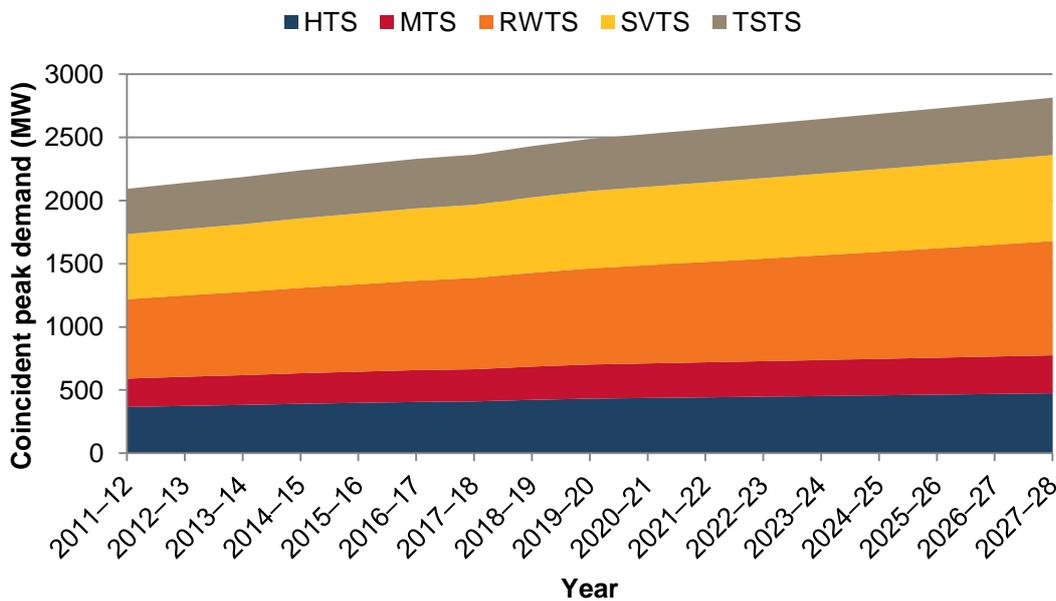
Figure 4 – Demand growth of stations supplied via Rowville No.1–No.2 220 kV bus group and Cranbourne
