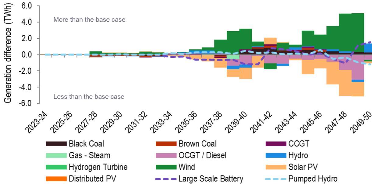
Figure 46 summarises the difference in generation and storage output forecast for Option 5 (in TWh), compared to the base case. These differences drive the avoided fuel cost benefit.
