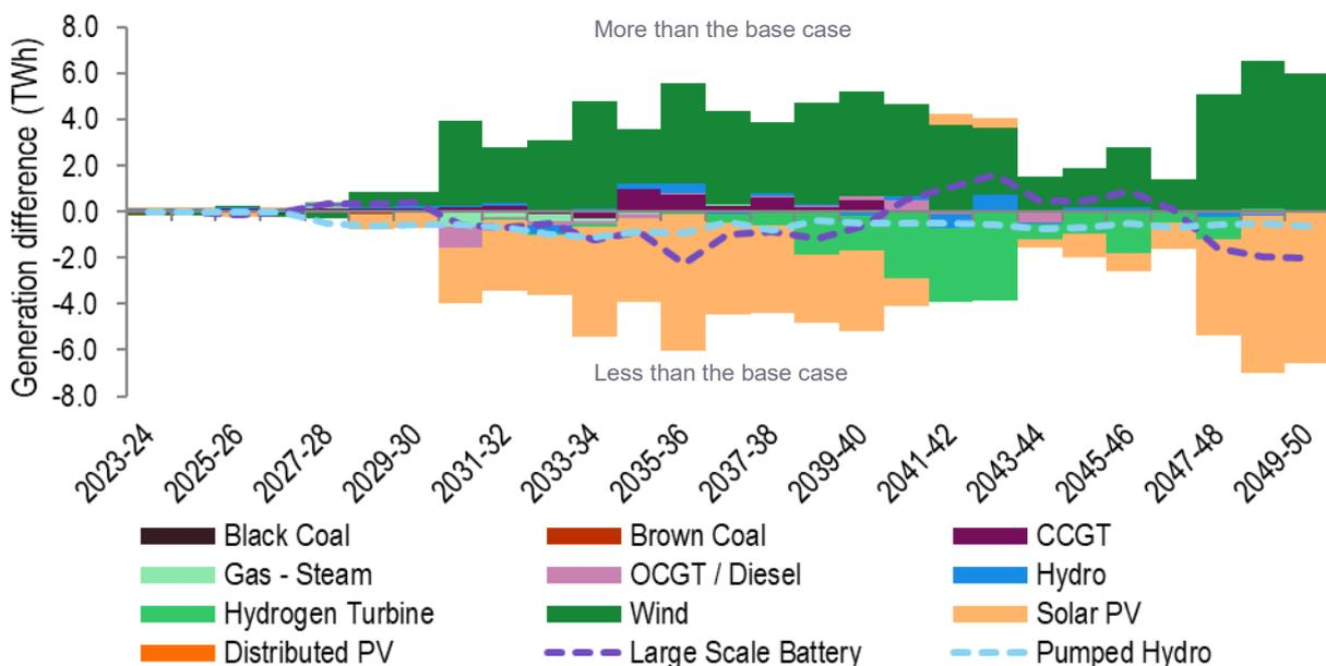
Figure 54 summarises the difference in generation and storage output forecast for Option 5 (in TWh), compared to the base case. These differences drive the avoided fuel cost benefit.
