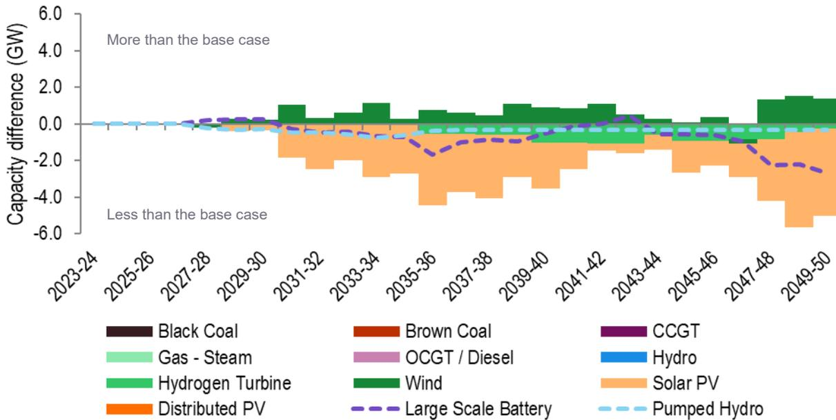
Figure 52 summarises the difference in generation and storage capacity forecast for Option 5 (in GW), compared to the base case. These differences drive the benefit associated with avoided or deferred generation and storage costs.
