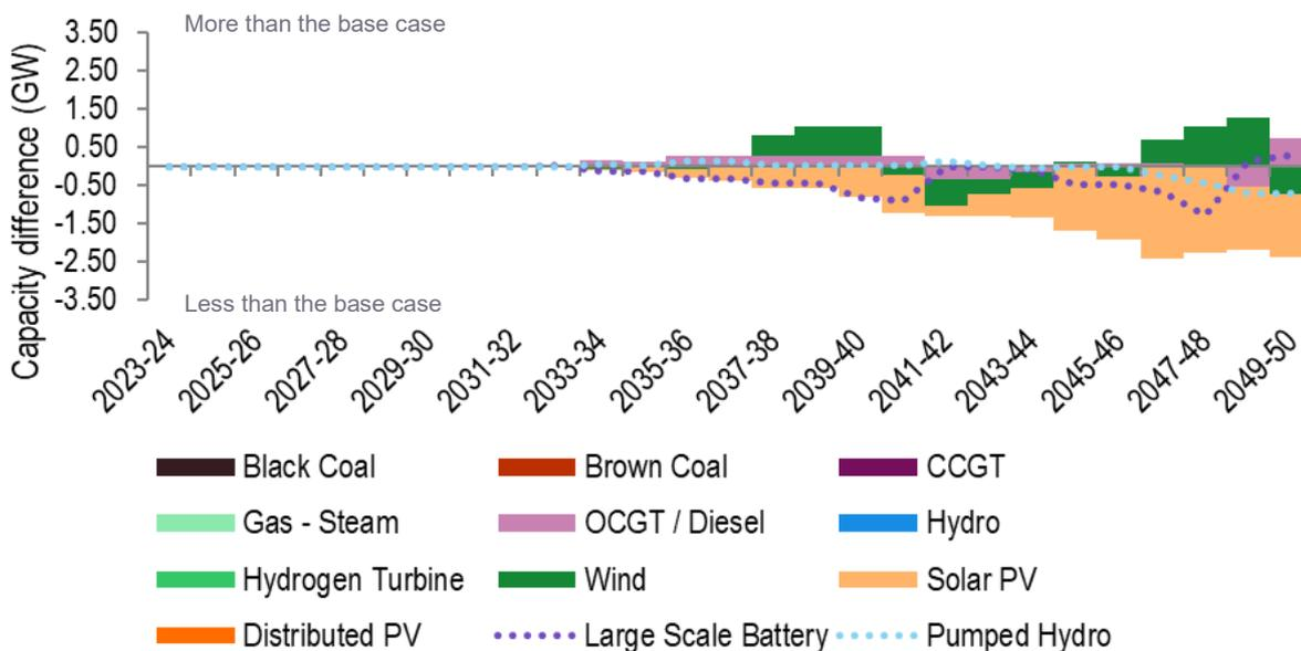
Similar to the *Step Change* scenario, in the *Progressive Change* scenario Option 3A is forecast to generally result in avoiding some solar and storage investment, though this option accelerates forecast wind and peaking gas build relative to the base case.
