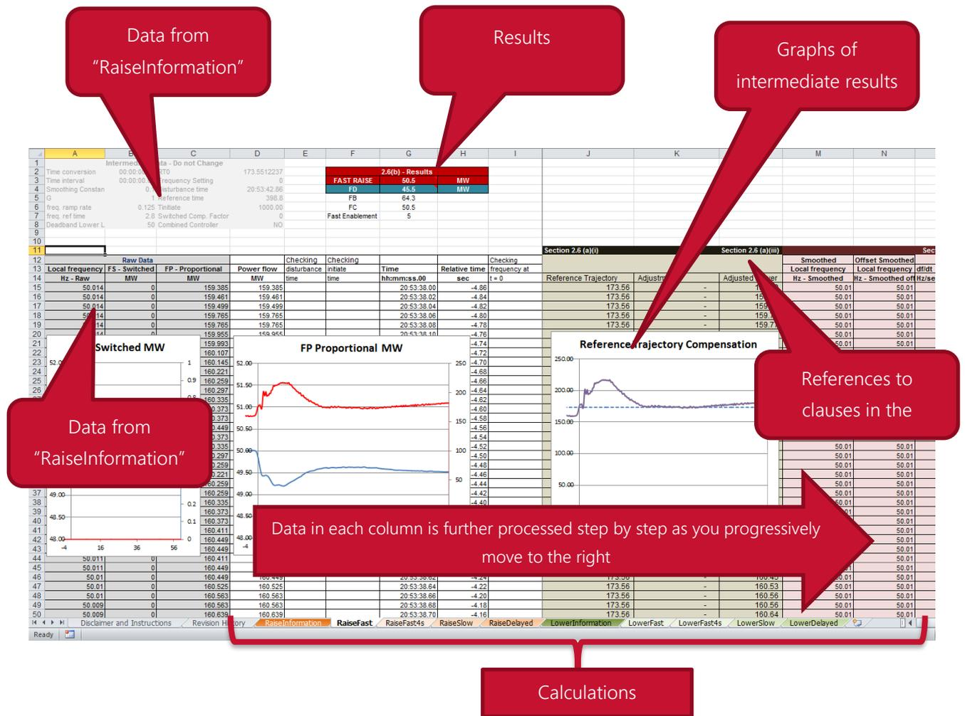
It can be seen that as the user moves progressively to the right, each column is further processed step by step as per the methodology in the MASS. The applicable clause numbers in the MASS are also identified to assist the user to locate the calculation step in the MASS. It is also instructive to consider the plots of intermediate results.
