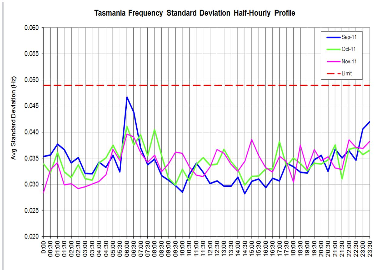
Figure 15: Daily profile of standard deviation for the frequency in Tasmania.
