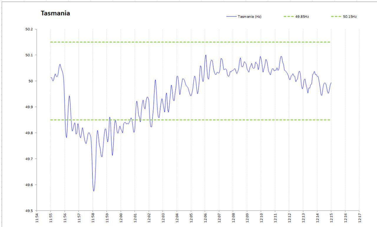
Figure 6: Tasmania frequency during low frequency generation event in Table 2 on 07<sup>th</sup> November 2011.
