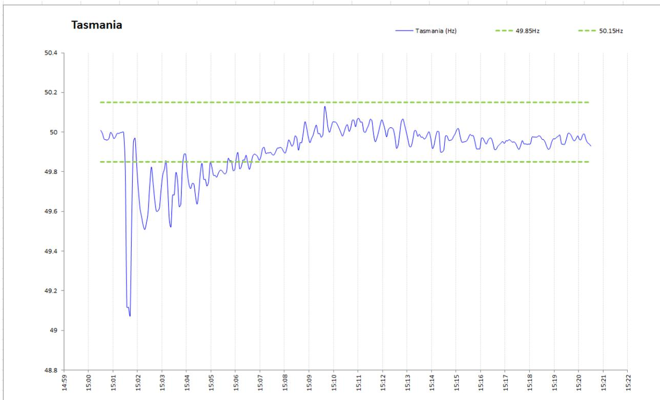
Figure 3: Tasmania frequency during low frequency generation event in Table 2 on 04<sup>th</sup> November 2011.
