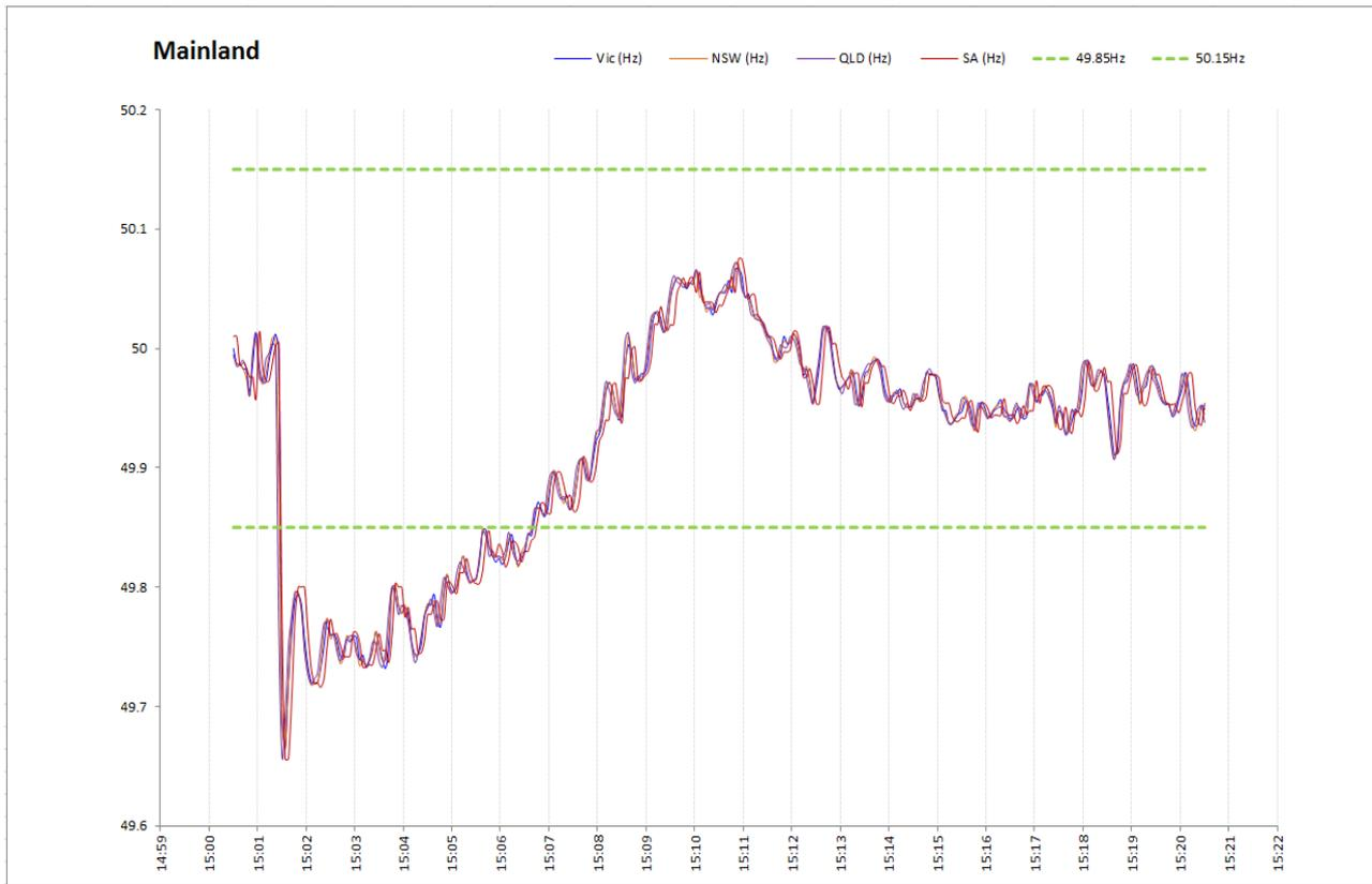
Figure 1: Mainland frequency during low frequency generation event in Table 2 on 04<sup>th</sup> November 2011.
