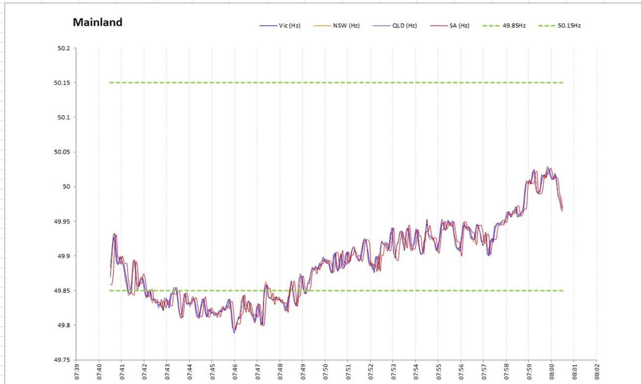
Figure 7: Mainland frequency during low frequency generation event in Table 2 on 29th November 2011
