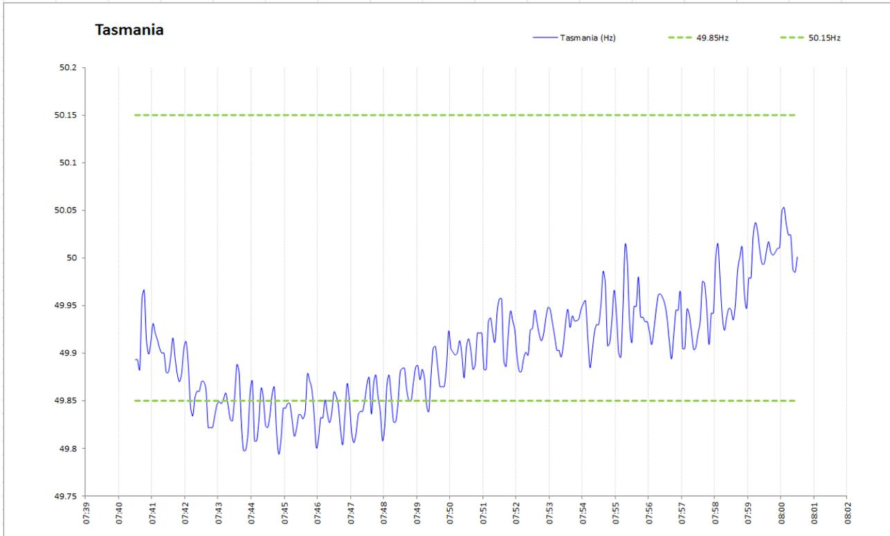
Figure 9: Tasmania frequency during low frequency generation event in Table 2 on 29<sup>th</sup> November 2011.
