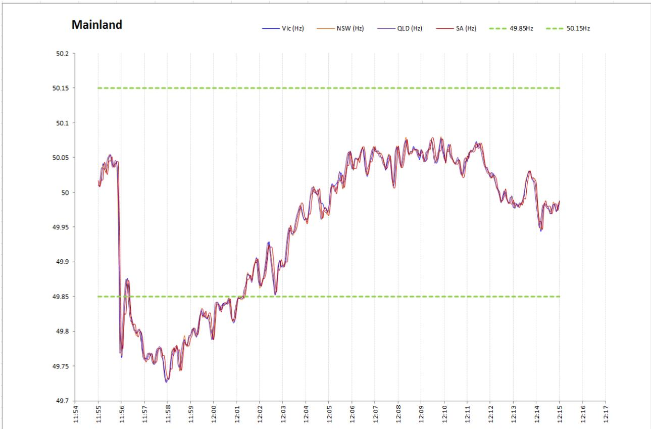
Figure 4: Mainland frequency during low frequency generation event in Table 2 on 07<sup>th</sup> November 2011.
