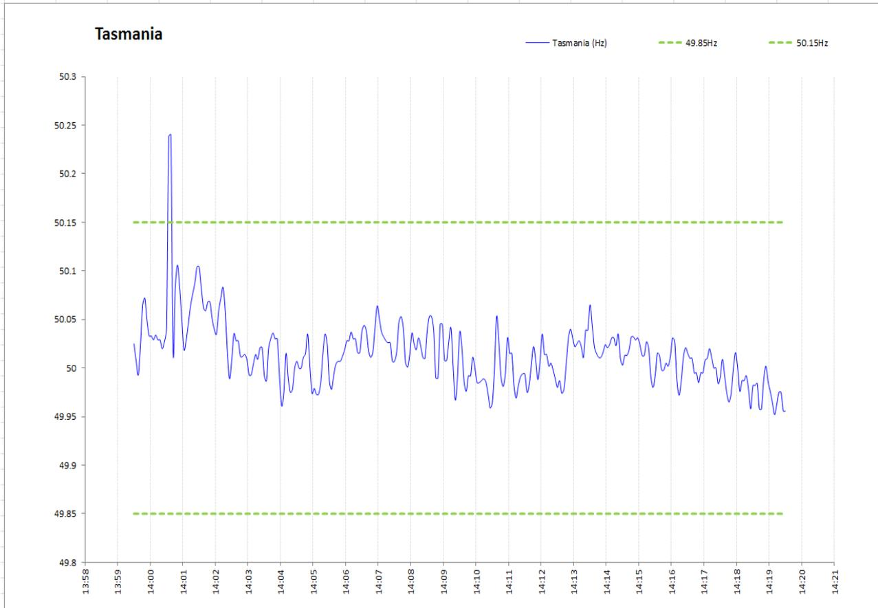
Figure 10: Tasmania frequency during High frequency No contingency event in Table 3 on 11<sup>th</sup> November 2011.
