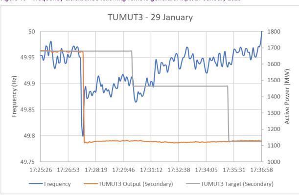
Figure 16 Frequency disturbance following TUMUT3 generator trips, 29 January 2023
