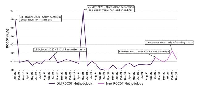
Note: 31 January 2020 RoCoF as measured in South Australia and 25 May 2021 RoCoF as measured in Queensland. New ROCOF calculation methodology used as of October 2022.
