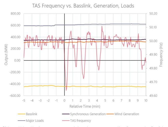
Of the two high and low frequency events recorded, one instance was caused by a flow reversal on Basslink on 27 January as shown in Figure 8. The second event occurred on 30 March while Basslink was cycling in and out of its 'no-go zone'.
