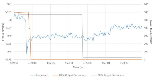
Figure 14 Frequency disturbance following Eraring Unit 4 generator trip
