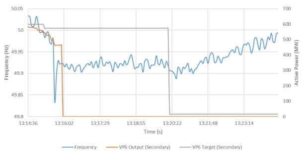
Figure 15 Frequency disturbance following VP06 generator trip
