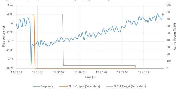
Figure 16 Frequency disturbance following KPP\_1 generator trip
