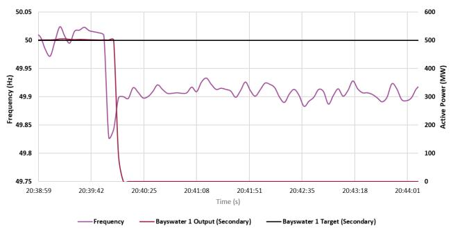
Figure 15 Frequency disturbance following Bayswater Unit 1 generator trip on 31 December 2023
