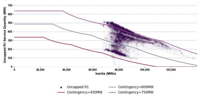
Figure 6 Relationship of uncapped L1 service quantities to inertia in Q4 2023
