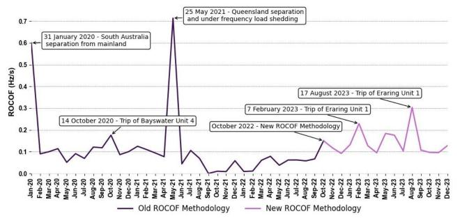
Note: 31 January 2020 RoCoF as measured in South Australia and 25 May 2021 RoCoF as measured in Queensland. New ROCOF calculation methodology used as of October 2022.
