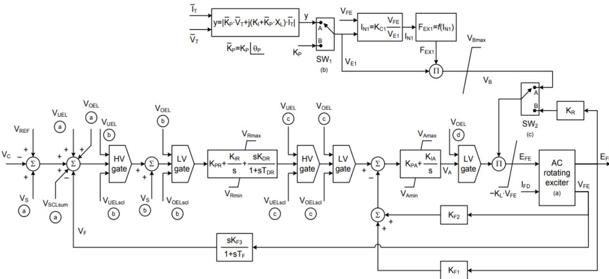
Figure 34 AC7B AVR excitation system based on IEEE 421.5-2005 ( $K_p = 0$  pu, PMG-fed independent AVR supply)
