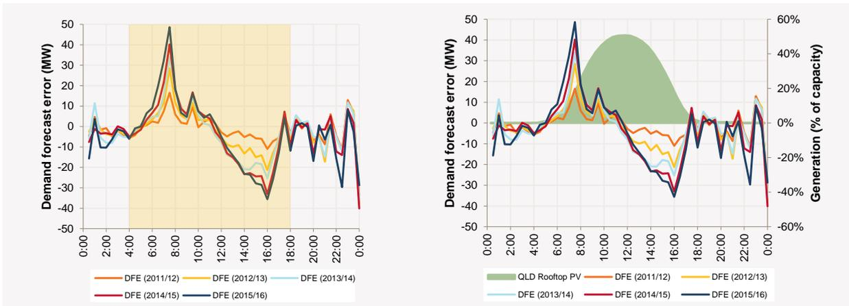
To investigate whether this is simply a coincidence, it can be compared to the change or ramping of rooftop PV generation rather than the generation output, as shown in Figure 8. This shows that the DFE is increasing proportionate to the change in solar generation.
