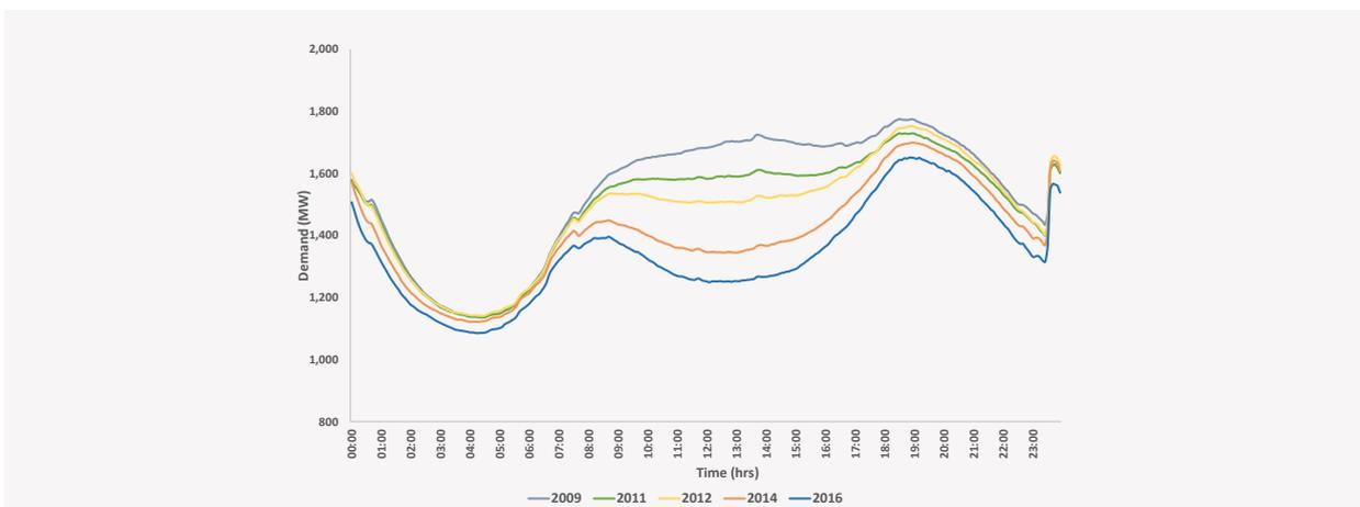
The figure shows the daily load profile based on averaged five minute data across selected calendar years between 2009 and 2016. As the capacity of rooftop PV has increased over the years, its impact on the load profile during the day is evident, with a large dip in demand followed by large ramping up in demand once the solar generation subsides.
