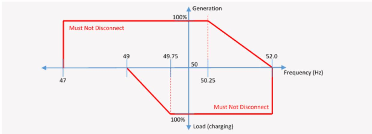
The introduction of the new AS/NZS 4777.2–2015 will result in the standardisation of frequency responses for PV inverters (including battery storage) compliant with the revised standard. This will mean that new compliant inverters will not disconnect for frequency disturbances in the range of 47 Hz – 52 Hz.
