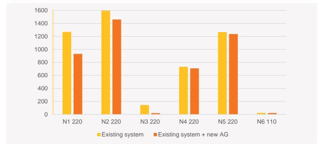
Figure 5 Assessment of available fault level at six Tasmanian busbar locations (new AG at N1 220)
