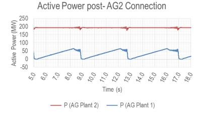
Figure 12 Dynamic behaviour of sub network post-AG2 connection
