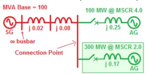
Consider the *connection point* shown in Figure 3 where an existing 100 MW AG is *connected*. A second AG (shaded) wishes to share the *connection point*.
