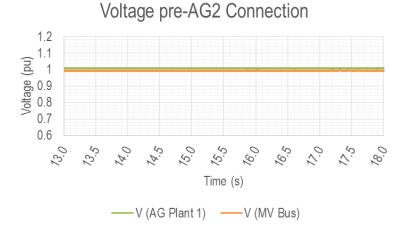
Figure 8 Dynamic behaviour of sub network pre-AG2 connection
