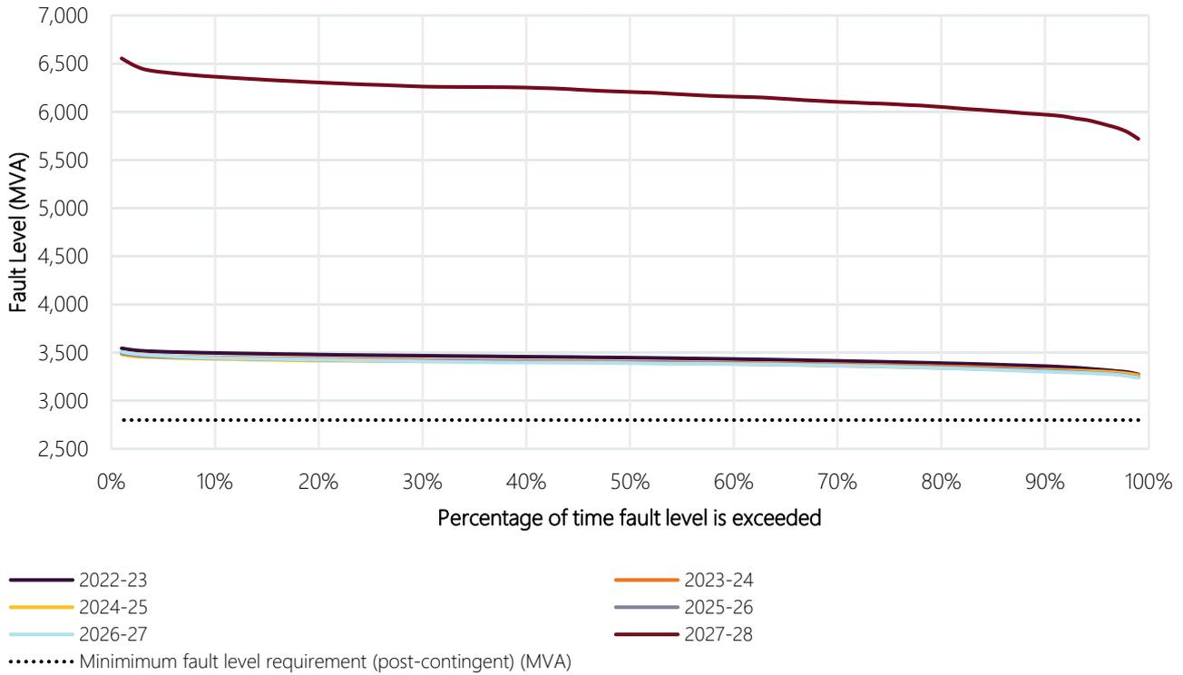
**Figure 8 Buronga node fault level duration curve<sup>A</sup>**
