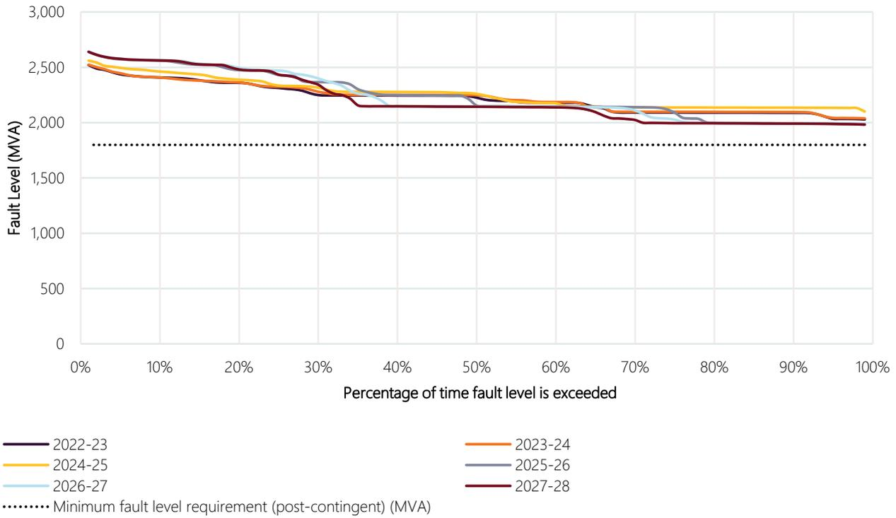
**Figure 25 Para node fault level duration curve against the minimum fault level requirement**
