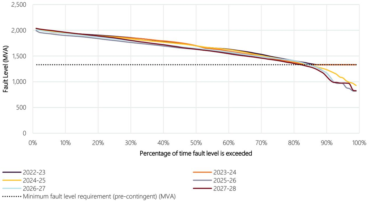
**Figure 32** Waddamana node fault level duration curve against the minimum fault level requirement
