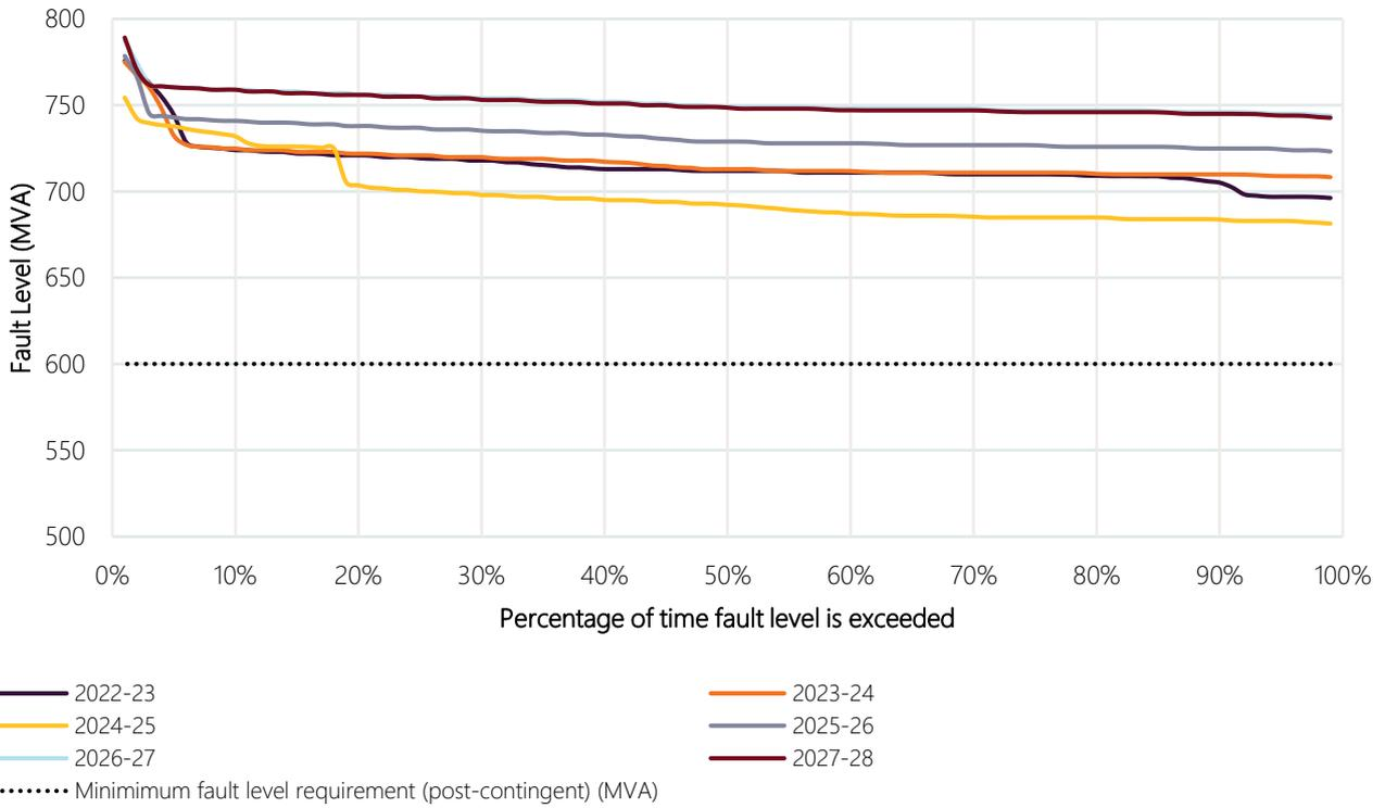
**Figure 10** Newcastle node fault level duration curve against the minimum fault level requirement
