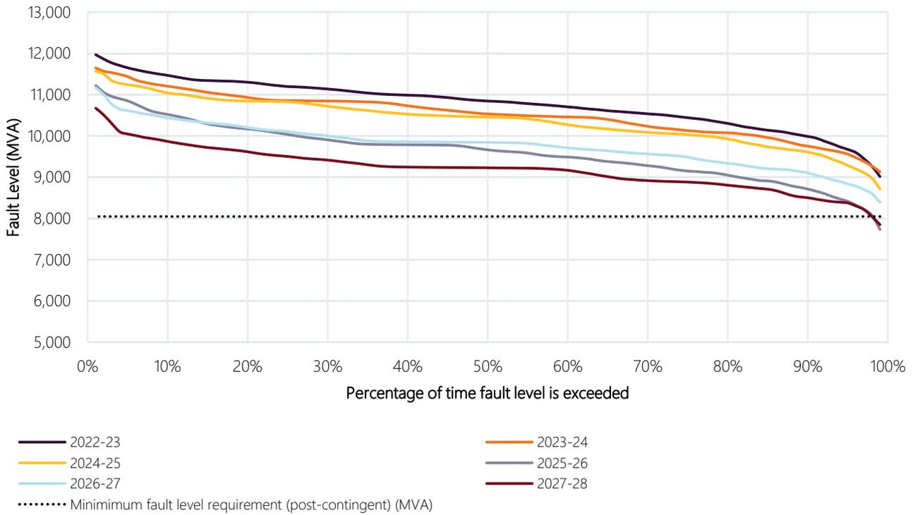
**Figure 12 Wellington node fault level duration curve against the minimum fault level requirement**
