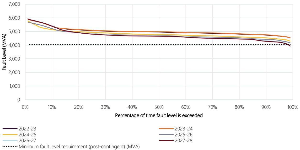
**Figure 39 Red Cliffs node fault level duration curve against the minimum fault level requirement**
