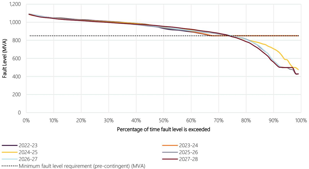
**Figure 30 George Town node fault level duration curve against the minimum fault level requirement**
