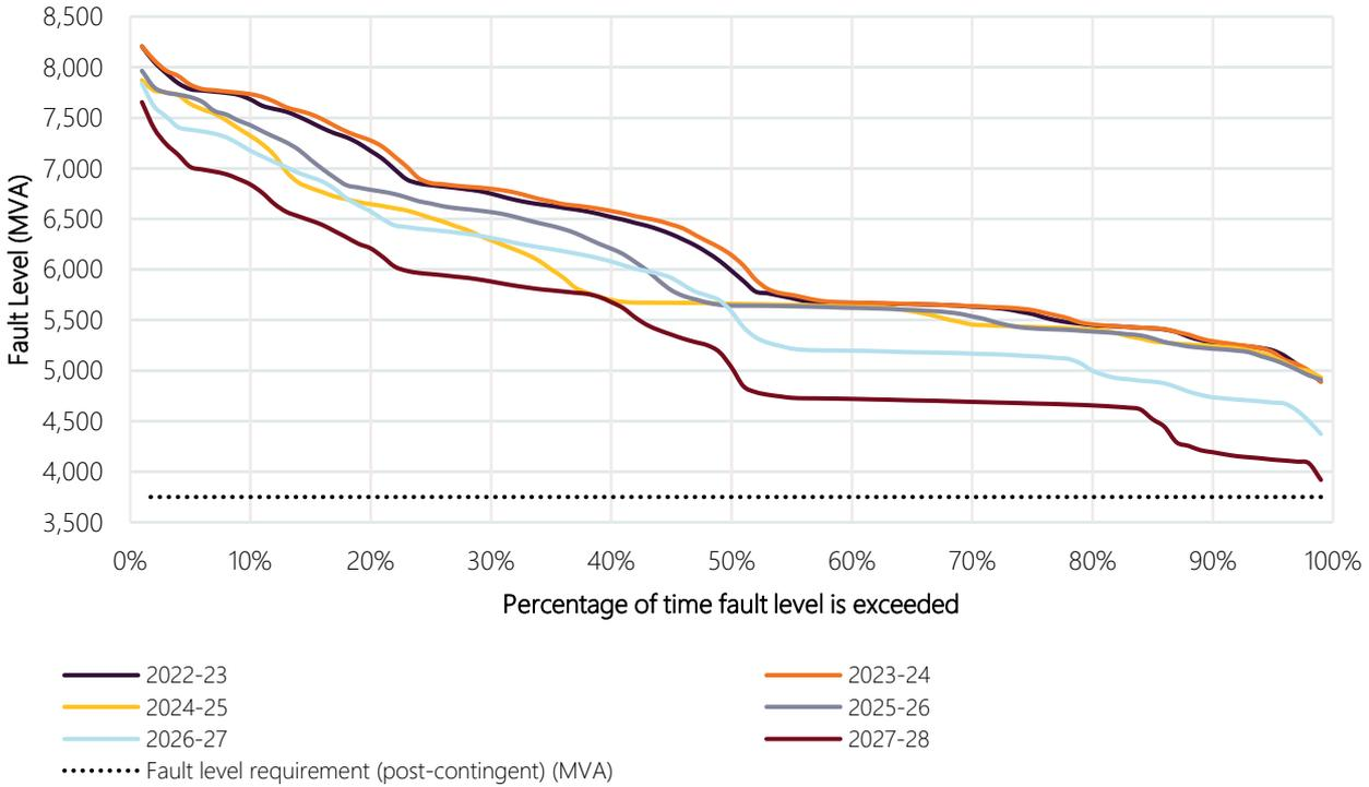
**Figure 19 Lilyvale node fault level duration curve against the minimum fault level requirement**
