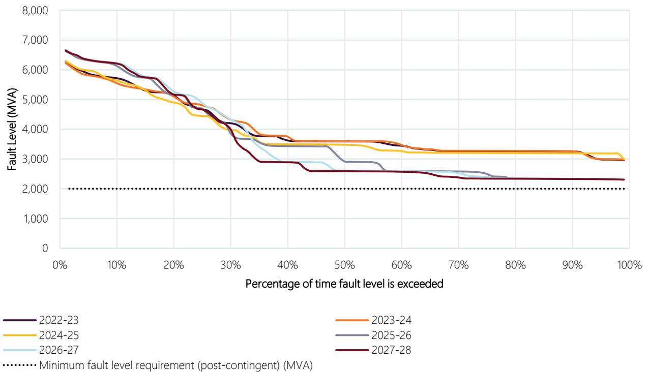
**Figure 26 Robertstown node fault level duration curve against the minimum fault level requirement**
