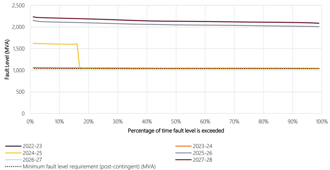
**Figure 40** Thomastown node fault level duration curve against the minimum fault level requirement
