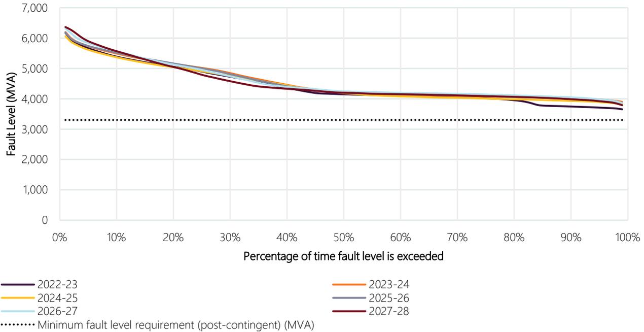
**Figure 37 Hazelwood node fault level duration curve against the minimum fault level requirement**
