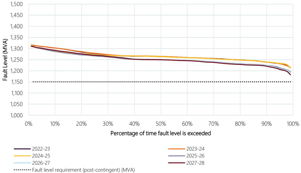
**Figure 20** Ross node fault level duration curve against the minimum fault level requirement
